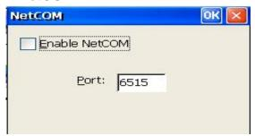
When enabled, another device on the network (using TELNET) can talk to a serial device (e.g. HyperTerminal) attached (null modem cable) to the ET com port. The SerialD type device is addressed on the network by the ET's IP address and Port 6515; e.g. OPEN 192.168.2.219 6515. Set mode to send CRLF (Carriage Return & Line Feed) when Enter is pressed (e.g. SET CRLF).
