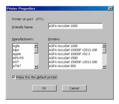
Select the manufacturer of your printer from **Manufacturers** list. Then, choose the desired printer model from **Printers** list. Give a specified name in Friendly Name field for the selected printer. Click check box of "**Make this the default printer**" to allow the selected one as default printer.
