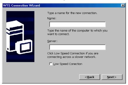
Type a name in Name field so a user can identify this RDP connection. Enter the name/IP address of the server in Server field. Check **Low Speed Connection** if using a Dialup network connection. Click **Next** to continue.
