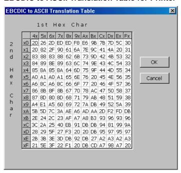
This table controls the EBCDIC to ASCII conversion for your printer session. You normally do not need to modify this table. If a character is printing on your printer with the wrong ASCII value, use the printer manual to determine the ASCII HEX value of this character and that of the value you want in its place. Find the incorrect value in the table, click on the value and type in the correct value. To exit this screen, click **OK**.
