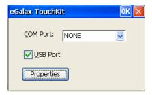
IMPORTANT NOTE: After you select the desired port, DO NOT click the Properties button. After you select the port, click OK, then reboot. After the reboot, you can select the Properties button to detect and calibrate your touch screen monitor. If you select Properties before a reboot, the user interface may hang.
