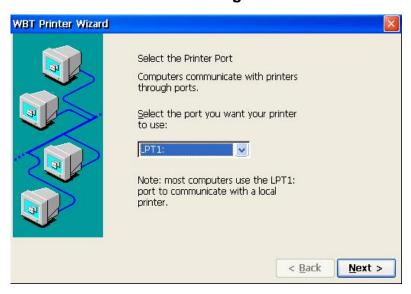
Select the port you want your printer to use. Most users select LPT1 port for a local printer. LPT2, if listed, represents a USB attached printer. COM1/COM2, if listed, refer to a serial attached printer.
