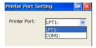
If **COM1** is selected, a **Port Setting** button is displayed in the above dialog. Clicking this button will display the **Com Port Setting** dialog as shown below.
