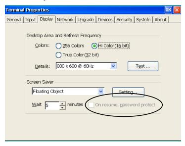
If enabled and checked when screen saver screen is exited, the user's password is requested as shown below.
