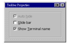
**Auto Hide**: Task bar is only shown when mouse cursor moved over bottom of the display (default). If not checked, the Taskbar is static at the bottom of the screen. To change this setting, first close all Connections.
