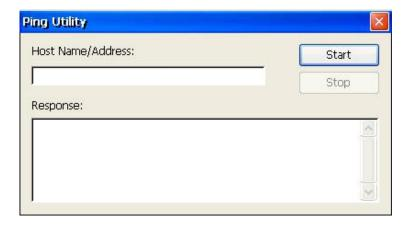
Enter Host name or IP address to ping. Click **Start** to ping the Host. A series of Pings will be sent to the Host. Click **Stop** button to end the process.
