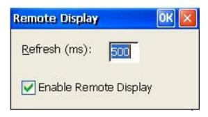
The Remote Display applet allows you enable or disable remote shadowing via the SNMPAdm Management tool. The refresh time (in milliseconds) affects the responsiveness and bandwidth utilization of the shadowing function. The lower the number, the faster the response and the more bandwidth used.
