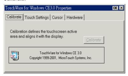
When the *Calibrate* button is active you can click it to calibrate the touch sensitivity and screen extent. You will get a screen with crosshairs in the lower left that you will touch for calibration, then touch the crosshairs in the upper right. After you are finished touch the "Done" button that appears in the Calibrate Complete screen.
