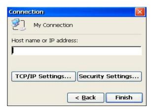
Enter name or IP address of the VPN server for the network to which you want to connect.
