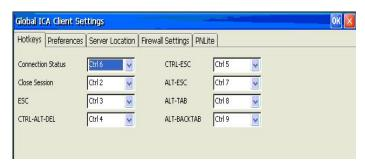
This dialog box is invoked through the **ICA Client Settings** tab found in the **Terminal Properties** dialog box. It is the default hotkeys properties sheet. To customize default hotkey key sequences, use the pull-down scroll boxes on the Hotkey properties. The following describes the function of Hotkeys.
