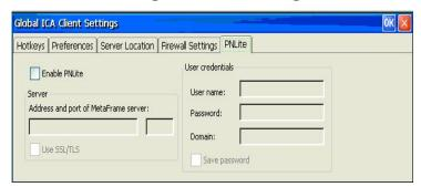
PNLite is an ICA connection mode that lets clients running CE 3 connect to Citrix server applications without having to configure connections for published applications. The names of such applications are added to the Terminal Manager Connection name list.
