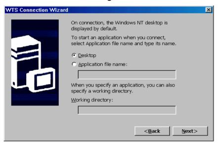
This dialog box allows you to access a desired application directly after connecting to the RDP server. The **Desktop** is the default. Click **Application File Name** to enter the name of the desired application and its working directory. Click **Next** to continue.
