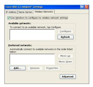
From within the **Wireless Network** tab, you can specify the type of wireless network in your environment. Businesses normally only use Access Point based networks. The default setting "Any available network (access point preferred)" is sufficient for most applications. You can specify "Access point (infrastructure) networks only" to add a layer of additional security if desired. The option "Automatically connect to non-preferred networks" is only
