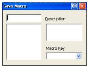
Enter the file name you want the macro saved as. Type the description of the macro for future reference. Assign the macro to a function key - required if keyboard used to Play back the macro.
