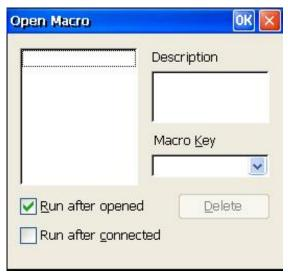
To automatically run a macro after the connection is started, select a macro from the list and check "**Run after connected"**.
