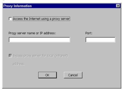
If your internet connection uses a proxy server, check the Access box and specify the Proxy server name or IP address and the Port number used.
