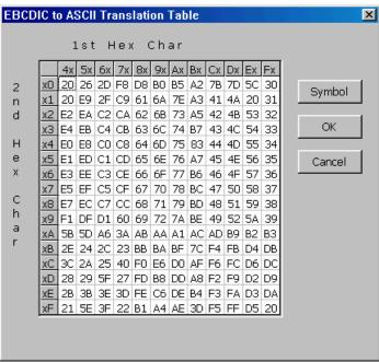
This table controls the EBCDIC to ASCII conversion shown on the display session. You normally do not need to modify this table. To modify the table, click on the ASCII value you want to change. You simply overwrite the default value by typing the new value. To exit this screen, click on **OK**.
