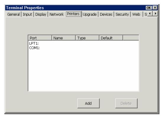
This dialog box allows you to setup a local printer for use by RDP connections. Select the Port to be used. Click **Add** to create a new local RDP printer. Click **Delete** to delete the current local printer.
