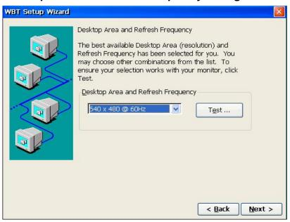
Select from the scroll list to set the resolution. The default setting is **800x600 (640x480) @ 60Hz**. Always click *Test* to see the resolution selected temporarily and determine whether it works with your monitor.
