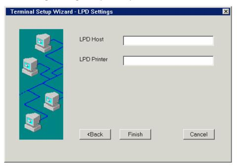
This dialog box is valid for TN3270 screen copy only. To enable this feature, enter LPD (Line Printer Daemon) Host IP address and queue name of the LPD printer in required fields.
