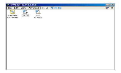
To configure a wireless connection on an ET5000, double click CISCO and refer to Chapter 11 for detailed procedures.
