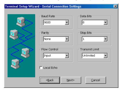
This dialog box only displays when ASCII session in Figure 6-1 and Serial connection in Figure 6-10 are selected. Enter the specific value or the default will be used.
