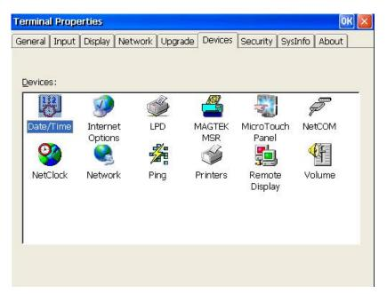
Special devices are supported by special modules referenced by this Tab. Double click the desired device setup icon. New device support may be added - check our home page (<a href="www.computerlab.com">www.computerlab.com</a>) for a description of any such devices.
