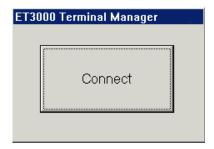
Special Connect Button escape sequence: Repeatedly click on the Connect button border to show the Terminal Properties screen. If Security is active and not signed on as Administrator, only the tabs General, Input, Display, Devices, SysInfo, and About will be available for use.
