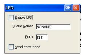
If you have a printer attached to the parallel printer port, you can make this printer a network printer. In this case, given the IP address of the WBT (see SysInfo) and the Queue Name, devices on the network can print to your attached printer.
