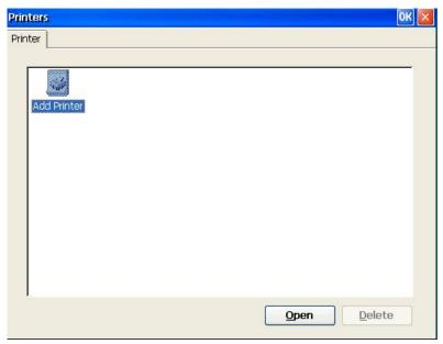
Click *Open* to setup a local printer. Click *Delete* to delete the local printer. Click *OK* to return to the Local Printer Setup dialog box.
