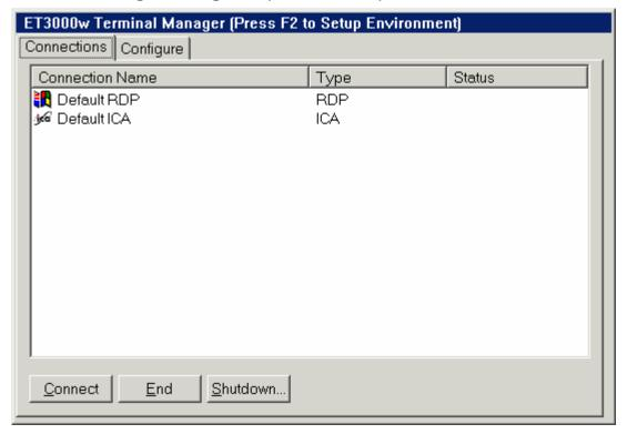
After you finish the initial terminal setup, the Terminal Manager dialog box will display. Unless Security is in effect, this will be the first dialog box after you power on the terminal.
