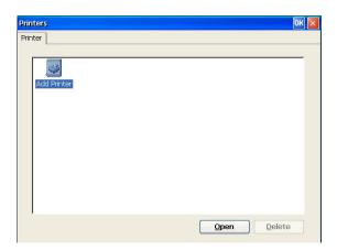
The Printers applet is used to define ICA and RDP printers. This user interface DOES NOT load a printer driver or in any way control local printers connected to the terminal. The only purpose for this applet is to "define" the local printer for a terminal server.
