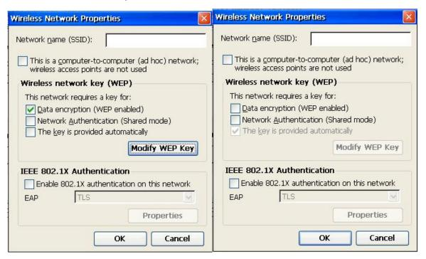
At the **Wireless (WEP) Key Settings** panel, enter the WEP key(s) used within your network. The key settings can be entered as hex or ASCII characters and accept values of 40 or 104 bits.
