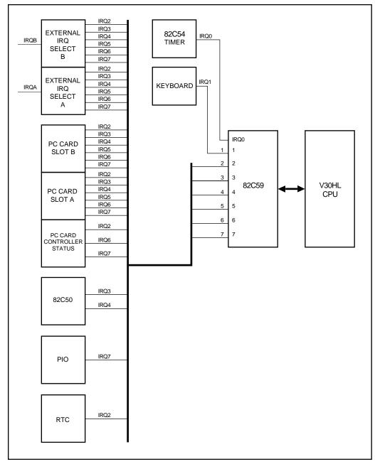
Two pins, IRQA and IRQB, provide support for the standard IRQ inputs. Each one of these inputs can support IRQ2-IRQ7. The selection of which IRQ input level is gated to the IRQA or IRQB inputs is controlled through the ICU mode register at index 0DH.
