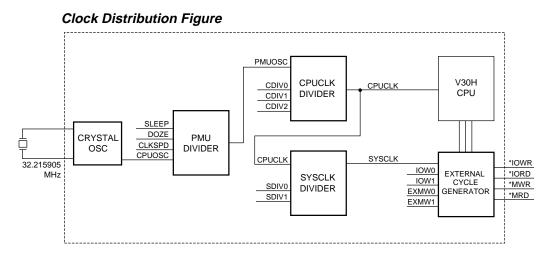
CPUCLK is derived from CPUOSC, and is configured through the BCG mode register at offset 01H. CDIV[2:0] select the divisor for CPUCLK. The default is CPUOSC/4.
