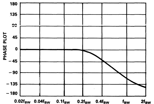
Figure 6. AD2S81A/AD2S82A Phase Plot
