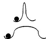
Figure 7. Triggering Modes of a Simple Flip-Flop
