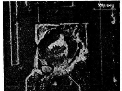
Fig.7 Enlarged micrograph of corroded Aluminum bonding pad
