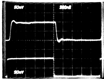
TOP TRACE: OUTPUT (50 mV/DIV AND 200 ns/DIV.) BOTTOM TRACE: INPUT (50 mV/DIV AND 200 ns/DIV.)
