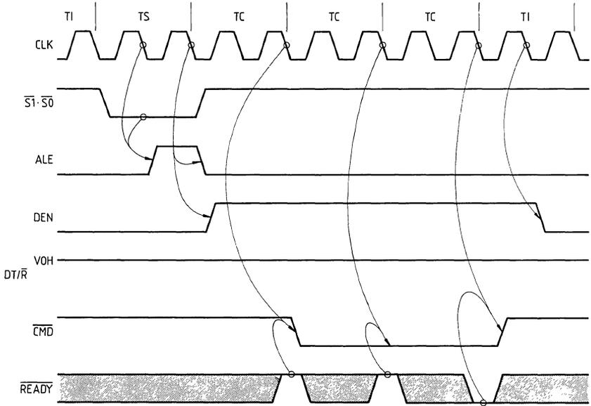
The MB control input affects the timing of the command and DEN outputs. These outputs are automatically delayed in Multibus mode to satisfy three requirements:
