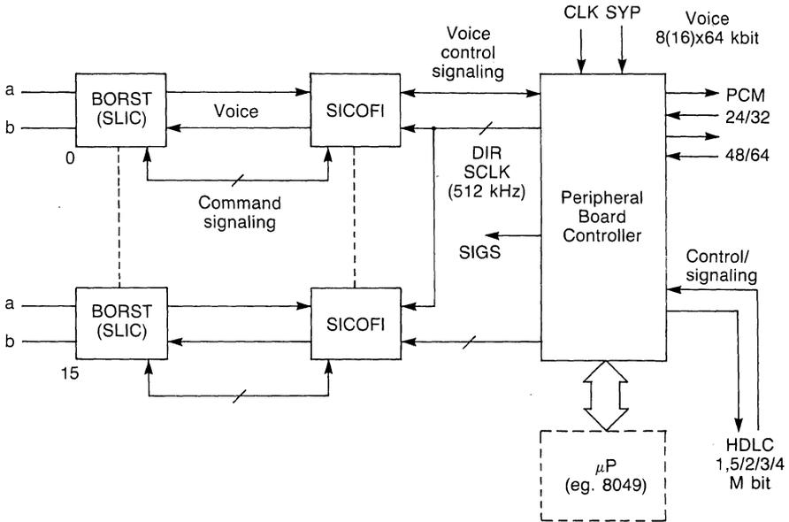
Fig. 1: Line Board Architecture
