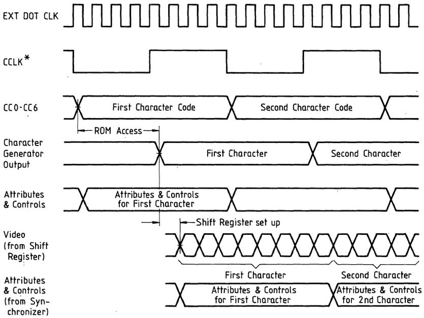
\*CCLK is a Multiple of the Dot Clock and an Input to the SAB8275
