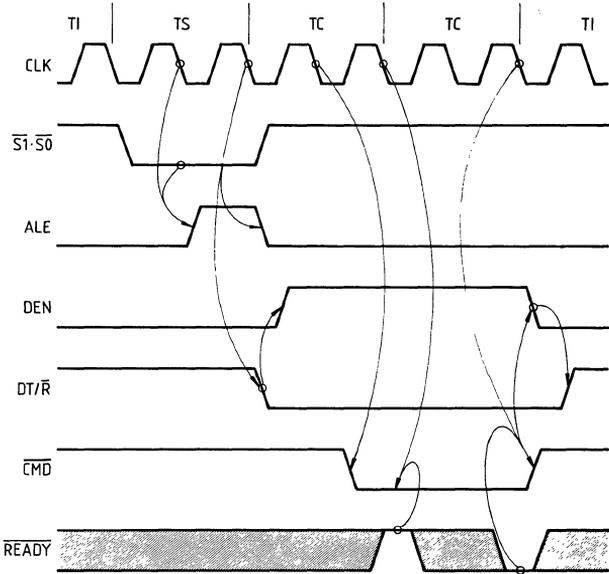
Idle-Write-Idle Bus Cycles with MB = 1
