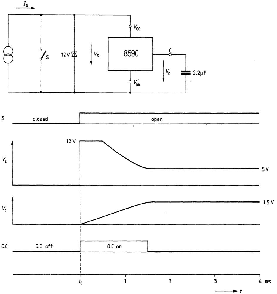
The control circuitry for the quick charging circuit has hysteresis with the following thresholds
