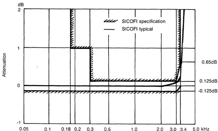
**ATTENUATION DISTORTION in RECEIVE DIRECTION**
