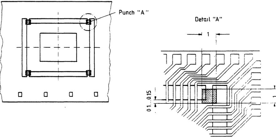
Lay down the punched MICROPACK onto an electrically conductive surface vacuum pickup.
