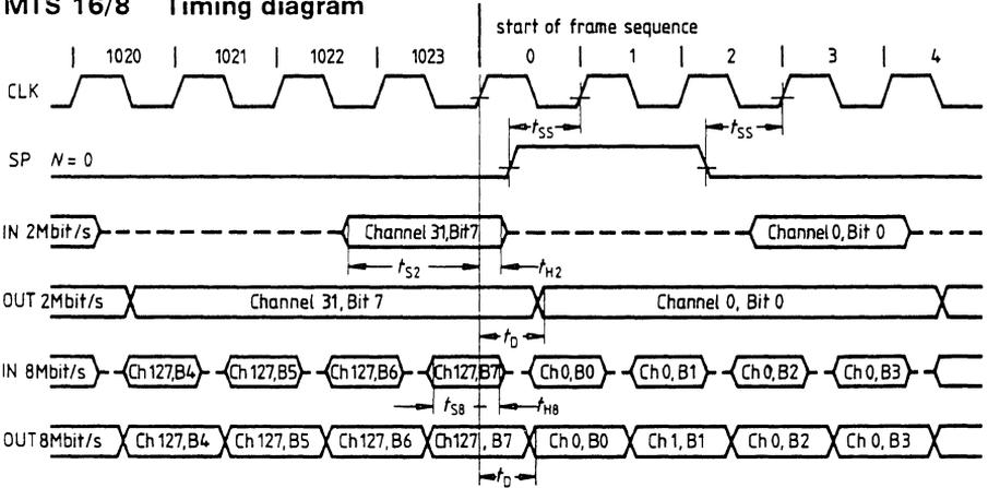
Example with delayed output frame
