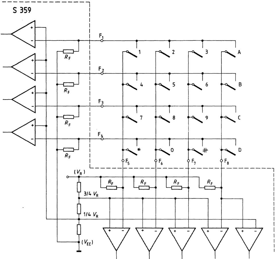
b) Electronic interface with a 2-of-8 keypad code
