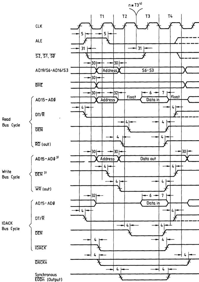
**Note 3:** For a Single Cycle Transfer the timing of AD15-AD0, DEN and DT/R is the same as in a Read Bus Cycle.
