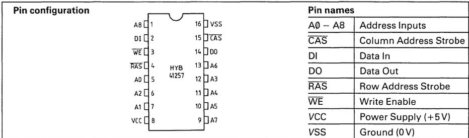
The HYB 41257 is a 262,144 word by 1-bit dynamic Random Access Memory. This 5V-only component is fabricated with Siemens new high performance N-channel silicon gate technology. The use of tantalum polycide provides high speed. A Siemens proprietary chip cover protects the chip against  $\alpha$  radiation.
