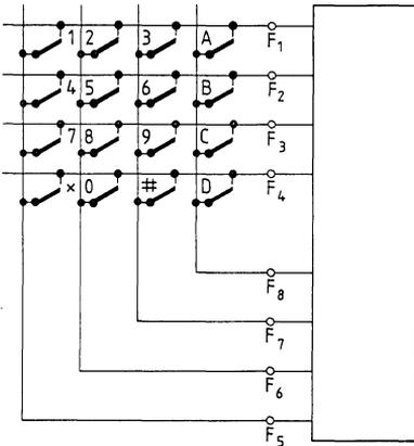
The keys are debounced and electronically interlocked. If more than one key is pressed simultaneously, the key recognized as pressed first will be evaluated.
