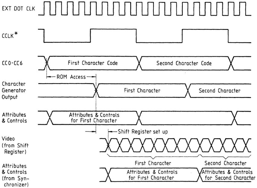
\*CCLK is a Multiple of the Dot Clock and an Input to the SAB 8276
