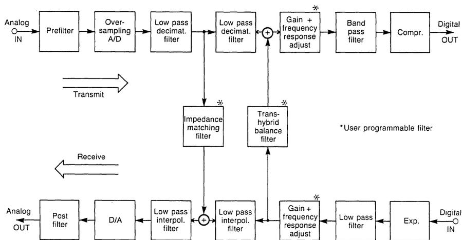
Fig. 2: Signal Flow
