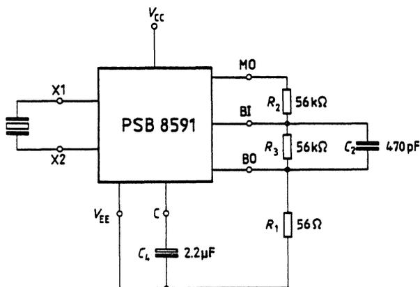
In order to keep the insertion loss for all the DTMF frequencies less than 0.2 dB the 3 dB cutoff frequency of the filter should be at least 6 kHz.
