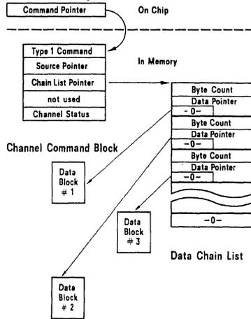
In the case of linked list chaining (see figure 13 a) each data block has a descriptor containing information on position of data block in memory, length of data block, and a pointer to the next description.
