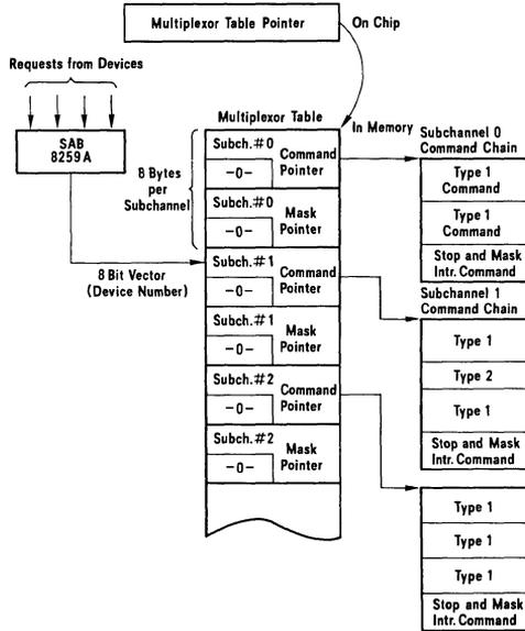
The mask pointer is the address of the appropriate SAB 8259A mask register.
