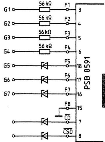
The enable inputs G5 to G7 have the following functions:
