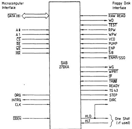
SAB 279XA is a floppy disk controller family of N-channel MOS LSI components designed to interface with SAB 8080/8051 family processors. Its flexibility and ease of use makes it an ideal floppy disk interface between conventional floppy disks and all computer systems. Software compatible with its predecessor, the SAB 179X, the device also contains a high performance Phase-
