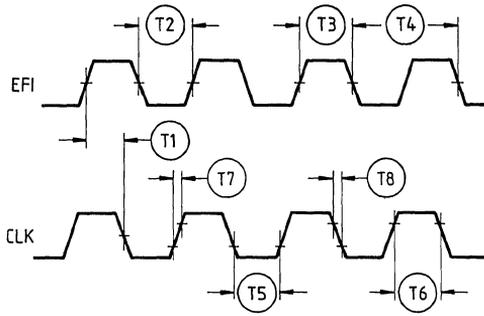
The EFI input LOW and HIGH times as shown are required to guarantee the CLK LOW and HIGH times shown.
