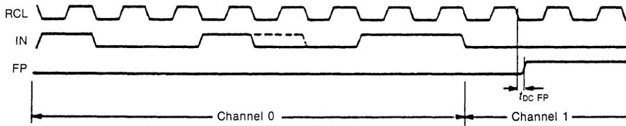
Delivery of fault pulse FP in the event of erroneous frame alignment signal
