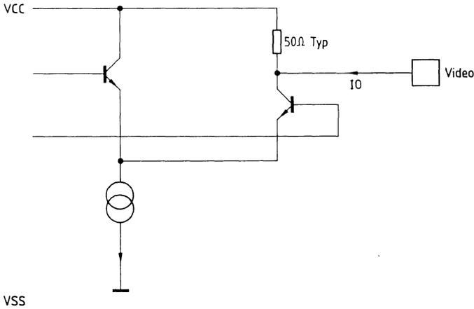
**Figure 14: Video Output Load**
