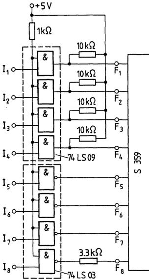
The inputs  $I_1$  to  $I_4$  control the frequencies of the lower frequency group  $f_1 - f_4$  and the inputs  $I_5$  to  $I_8$  control the frequencies of the higher frequency group. For the generation of a dual tone, one input of  $I_1$  to  $I_4$  of the lower group and one input of  $I_5$  to  $I_8$  of the higher group must have an H-level.
