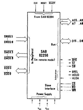
As a result of this, a bus compatibility with identical timing is attained with processors SAB 80286, SAB 80186 and SAB 8086. A compatibility with the 8 bit bus versions of these processors SAB 8088 and SAB 80188 is also guaranteed by defining the
