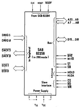
SAB 82258 is an advanced DMA (Direct Memory Access) Controller designed especially for the 16 bit microprocessors SAB 80286 and SAB 8086/186/88/188. In addition, the operation with other processors is supported by the remote mode. It has 4 independent DMA channels which can transfer data at rates up to 8 Mbytes/second at 8 MHz
