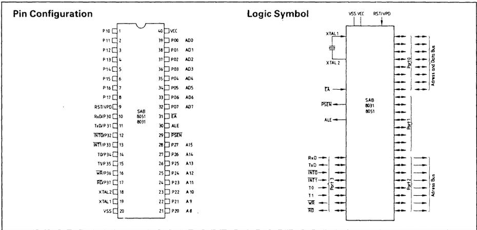
The SAB 8031/8051 is a stand-alone, high-performance single-chip computer fabricated in +5V advanced N-channel, silicon gate Siemens MYMOS technology and packaged in a 40-pin DIP. It provides the hardware features, architectural enhancements and new instructions that are necessary to make it a powerful and cost effective controller for applications requiring up to 64K bytes of program memory and/or up to 64K bytes of data storage.
