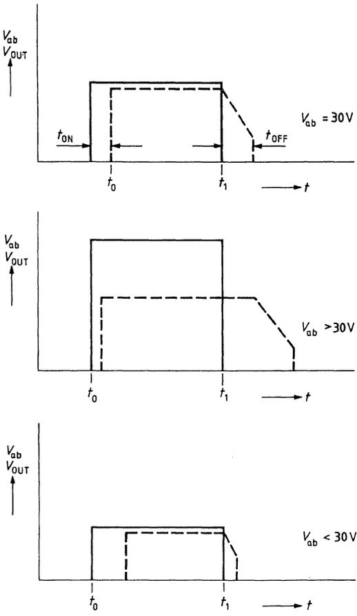
———— Effective value of input signal (call voltage  $V_{ab}$ )
