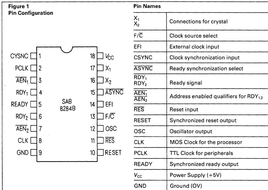
SAB 8284B is a bipolar clock generator/driver designed to provide clock signals for SAB 8086 and SAB 8088 processors and peripherals. It also contains READY logic for operation with two bus systems and provides the processors required
