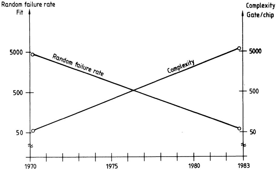
Figure 2 shows the general course of the failure rate for digital MOS ICs in fit for the years 1970 to 1983. The increasing complexity as regards gate functions/chip is also specified.
