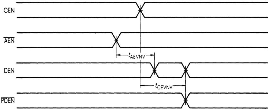
Address Enable (AEN) Timing (3-State Enable/Disable)
