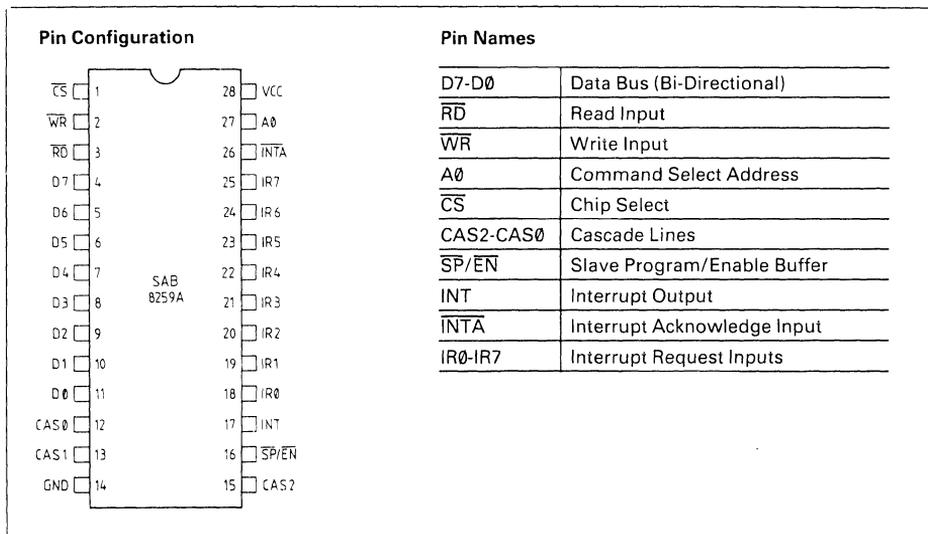
SAB 8259A Programmable Interrupt Controller handles up to eight vectored priority interrupts for the CPU. It is cascadable for up to 64 vectored priority interrupts without additional circuitry. It is packaged in a 28-pin DIP, uses NMOS technology and requires a single +5 V supply. Circuitry is static, requiring no clock input.
