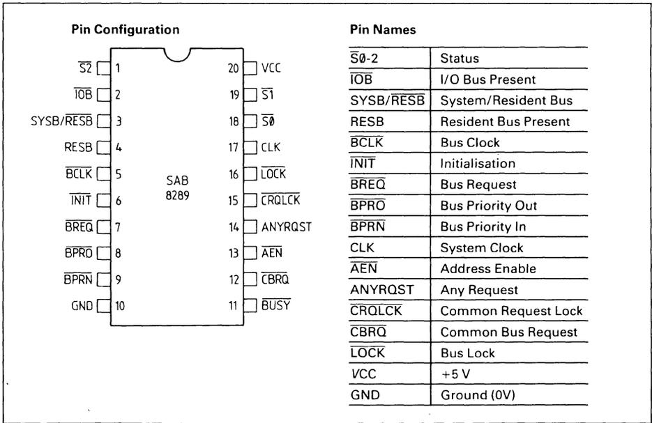
The SAB 8289 Bus Arbiter is a 20-pin, 5-volt-only bipolar component for use with medium to large SAB 8086/SAB 8088 multi-master/multiprocessing systems. The SAB 8289 provides system bus
