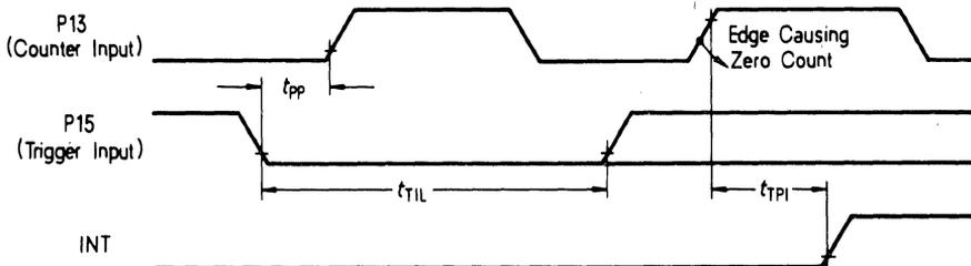
**Trigger Pulse for Timer 5 (Cascaded Event Counter/Timer 3 and 5)**
