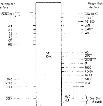
SAB 179X is a floppy disk controller family of N-channel MOS LSI components designed to interface with SAB 8080/8085/8086/8051 family
