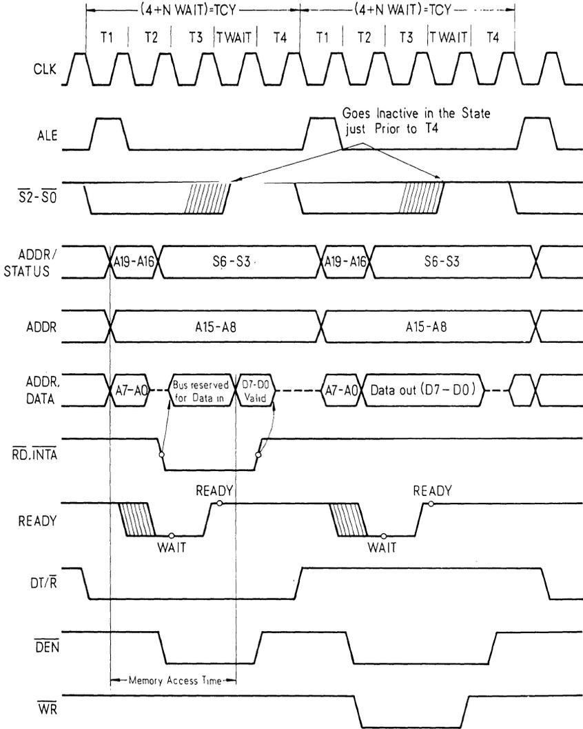
Status bits  $\overline{S0}$ ,  $\overline{S1}$ , and  $\overline{S2}$  are used by the bus controller, in maximum mode, to identify the type of bus transaction according to the following table:
