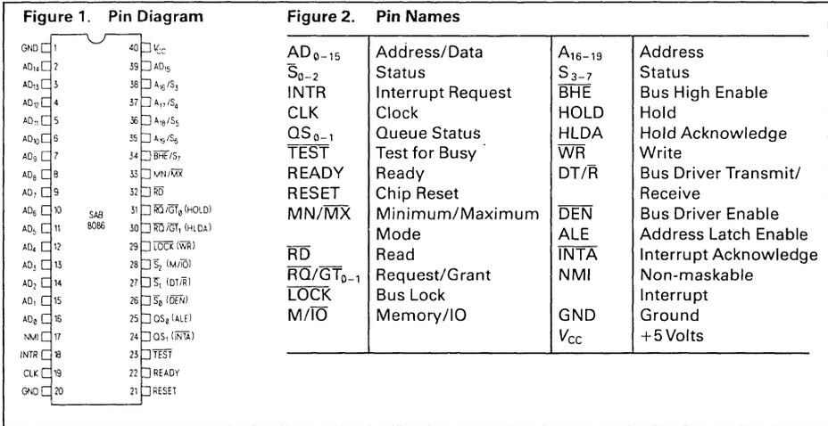
SAB 8086 is a new generation, high performance 16-bit Microprocessor implemented in +5 Volts, depletion load, N channel, silicon gate Siemens MYMOS technology packaged in a 40 pin package. It is 100 percent compatible with the industry
