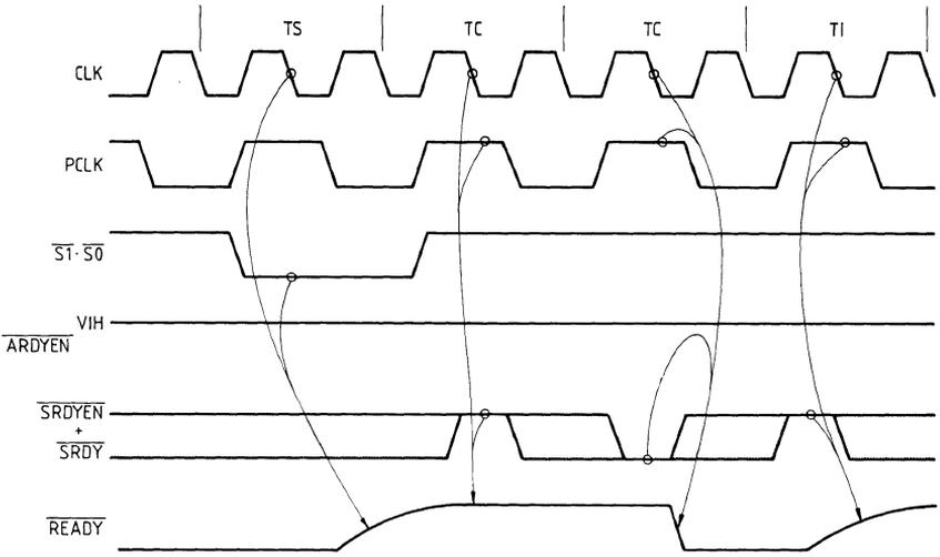
**Asynchronous Ready Operation**
