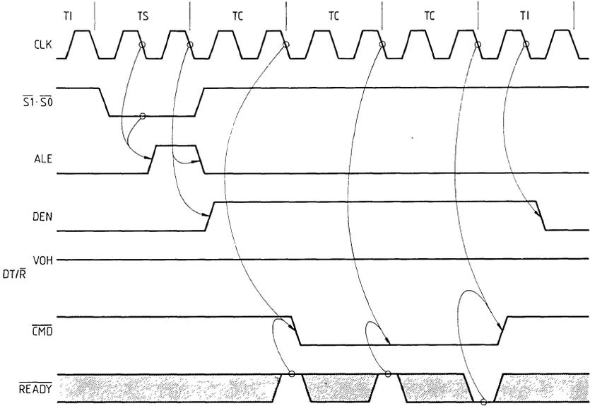
**Write-Write Bus Cycles with MB = 0**
