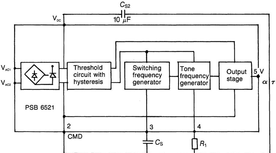
The IC contains an oscillator which generates a square wave voltage. The frequency of this voltage is periodically switched by a second oscillator back and forth between two basic values having a ratio of 1 : 1.25. The basic frequency  $f_{TR}$  is adjusted by the resistor  $R_T$  and the switching frequency  $f_s$  by the capacitor  $C_s$  (Figs. 12 and 13).
