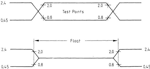
A.C. testing inputs are driven at 2.4V for a logic "1" and 0.45V for a logic "0".
