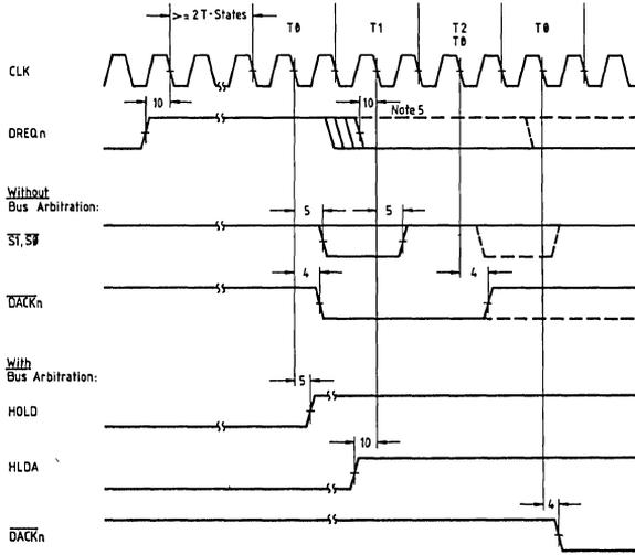
**Note 5:** The trailing edge of DREQ<sub>n</sub>, as specified in this diagram, is necessary if only one bus cycle should be executed.
