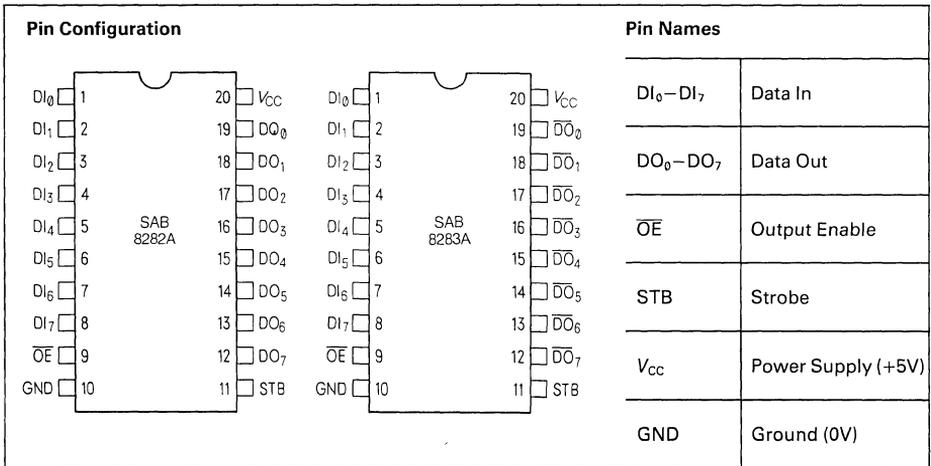
The SAB 8282A and SAB 8283A are 8-bit bipolar latches with 3-state output buffers. They can be used to implement latches, buffers, or multiplexers. The SAB 8283A inverts the input data at its outputs while the SAB 8282A does not.
