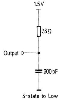
Test Load Circuits – 3-State Command Output Test Load
