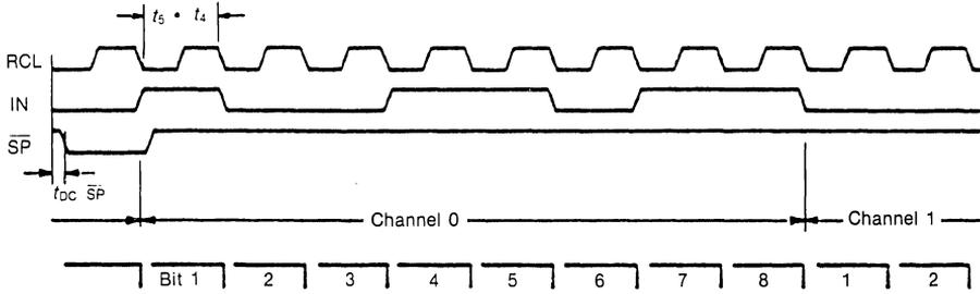
Delivery of synchronous pulse  $\overline{SP}$  in synchronized state
