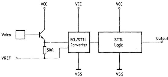
Figure 15: Proposed Converter for Video Output to TTL Level Output
