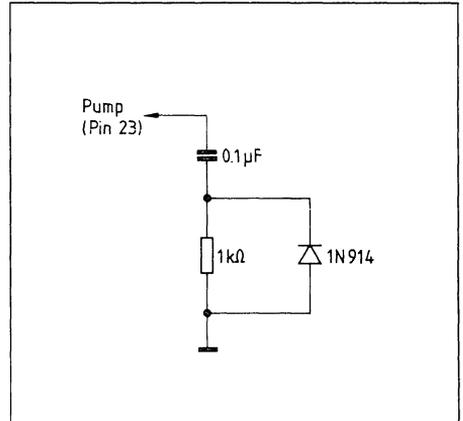
Since  $5\frac{1}{4}$ " Drives operate at exactly one-half the data rate (250 Kbytes/sec) the above capacitor should be doubled to 0.2 or 0.22  $\mu\text{F}$ .
