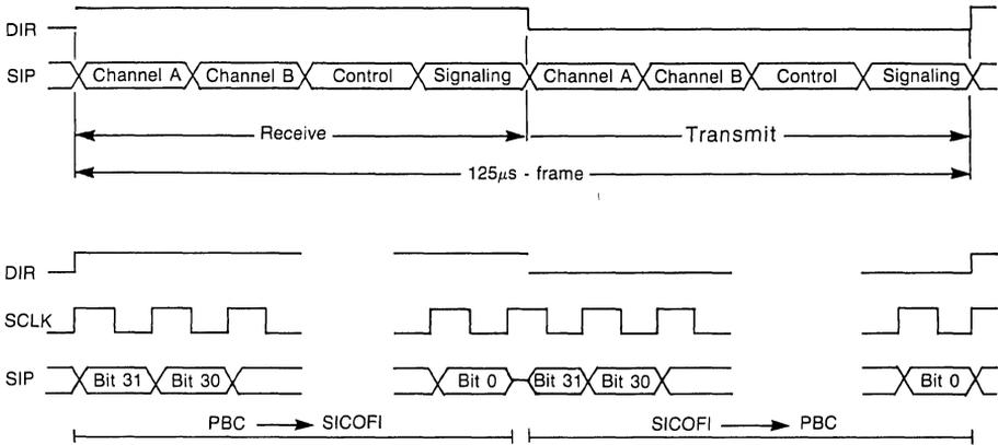
Fig. 4: Byte sequence and timing at Serial Interface Port SIP
