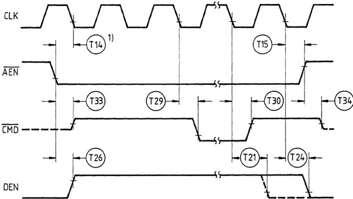
1)  $\overline{AEN}$  is an asynchronous input.  $\overline{AEN}$  setup and hold time is specified to guarantee the response shown in the waveforms.
