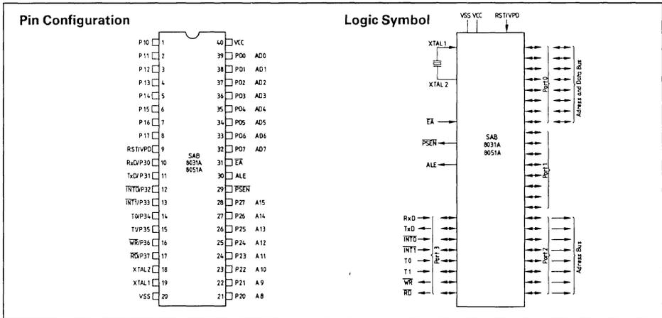
The SAB 8031A/8051A for the two extended temperature ranges (Industrial temperature range:  $-40$  to  $+85^{\circ}\text{C}$ , Automotive temperature range:  $-40$  to  $+110^{\circ}\text{C}$ ) is fully compatible with the standard SAB 8031A/8051A with respect to architecture, instruction set, and software portability.
