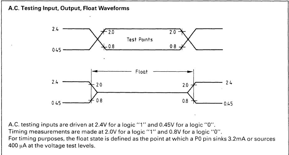
A.C. testing inputs are driven at 2.4V for a logic "1" and 0.45V for a logic "0".
