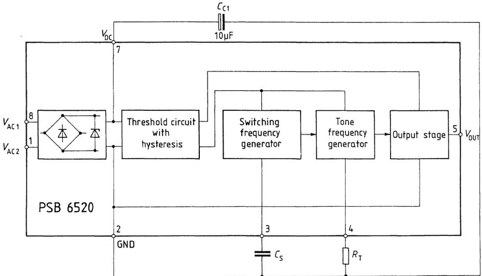
The IC contains an oscillator which generates a square wave voltage. The frequency of this voltage is periodically switched by a second oscillator back and forth between two basic values having a ratio of 1 : 1.38. The basic frequency  $f_{1T}$  is adjusted by the resistor  $R_T$  and the switching frequency  $f_S$  by the capacitor  $C_S$  (**fig. 12 and 13**).
