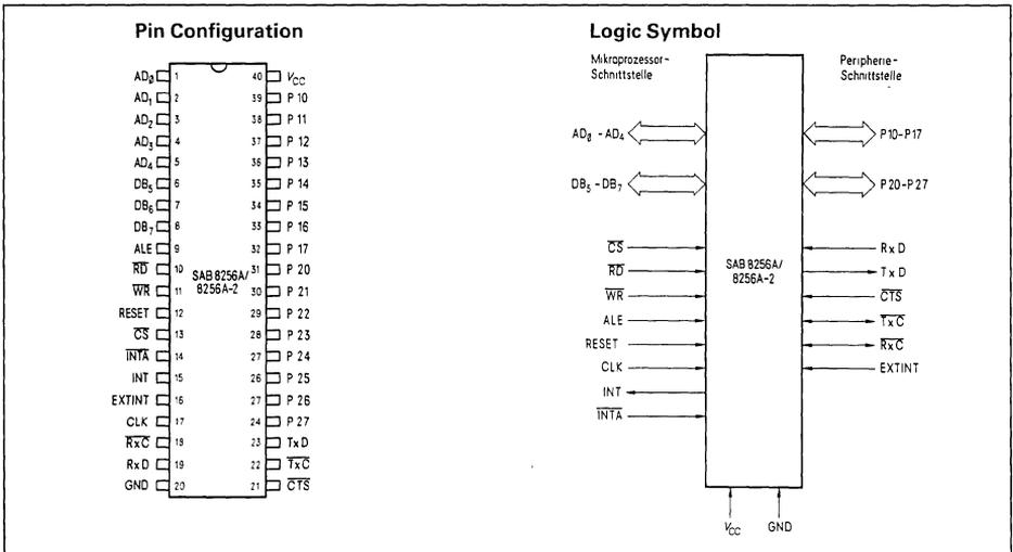
SAB 8256A integrates four of the most used peripheral functions in a microcomputer system into a 40 pin package: serial interface, parallel interface, timer/counter and interrupt controller. It is primarily suited for system like SAB 8048, SAB 8085, SAB 8086, SAB 8088, SAB 80186 and
