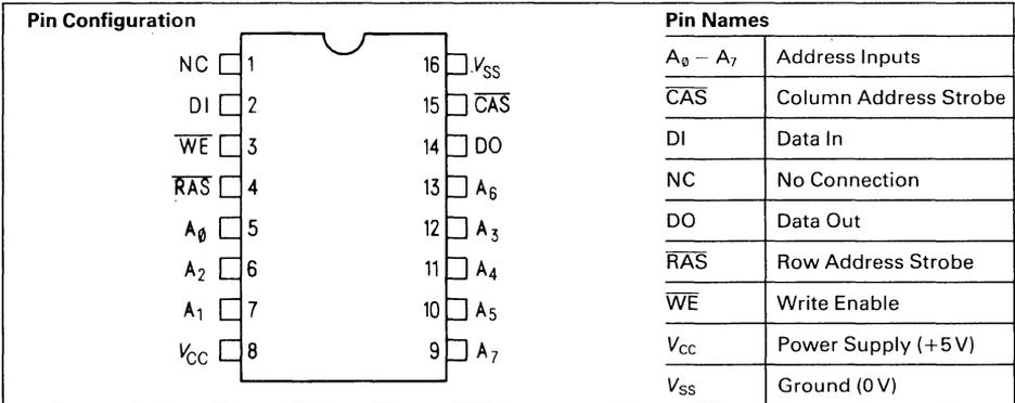
The HYB 4164 is a 65536-word by 1-bit, MOS random access memory circuit fabricated with Siemens new 5-Volt only n-channel silicon gate technology, using double layer polysilicon. To protect the chip against  $\alpha$ -radiation a Siemens proprietary chip cover is used. The HYB 4164 uses single transistor dynamic storage cells and dynamic control circuitry to achieve high speed at very low power dissipation.
