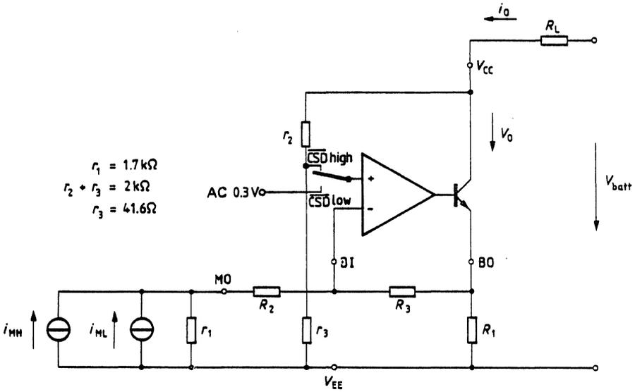
The internal feedback loop is normally closed ( $r_2$ ,  $r_3$ , positive input of output amplifier). If the current sink is disabled, the positive input of the output amplifier is supported with a fixed voltage of about 0.3 V. This voltage is derived from the internal reference voltage.
