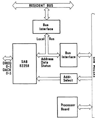
SAB 82258 has four independent DMA channels that can transfer up to 8 Mbytes/sec in the single cycle mode (2 clocks/transfer). In the 2 cycle transfer mode the maximum rate is 4 Mbytes/sec. Switching between channels induces no time penalty. Thus the overall maximum transfer rate of
