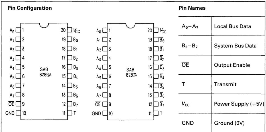
The SAB 8286A and SAB 8287A are 8-bit bipolar transceivers with 3-state outputs. The SAB 8287A inverts the input data at its outputs while the SAB 8286A does not. Thus, a wide variety of applications for
