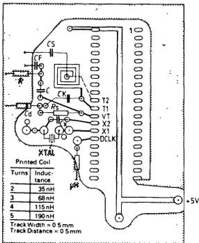
e) example layout for printed circuit
