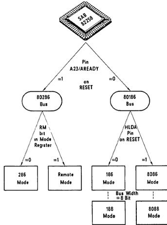
SAB 82258 can also operate in a remote or stand alone mode where it is not coupled directly to a processor. Figure 5 shows the way how SAB 82258 detects with which processor or in which mode it is operating. Figure 2 shows the logic pinning in the 286 mode – for operation with SAB 80286. Figure 3 shows the logic pinning in the 186 mode – for operation with SAB 80186/188 and SAB 8086/88, and Figure 4 shows the pinning when SAB 82258 is in the remote mode and not directly coupled to a processor.
