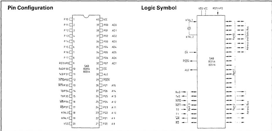
The SAB 8031A/8051A is a stand-alone, high-performance single-chip computer fabricated in +5V advanced Siemens MYMOS technology and packaged in a 40-pin DIP. It provides the hardware features, architectural enhancements and new instructions that are necessary to make it a powerful and cost effective controller for applications requiring up to 64 Kbytes of program memory and/or up to 64 Kbytes of data storage.
