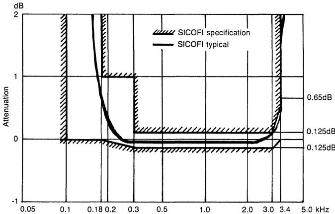
**ATTENUATION DISTORTION in TRANSMIT DIRECTION**
