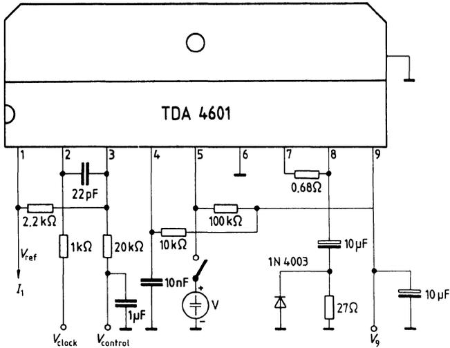
Test diagram: overload operation
