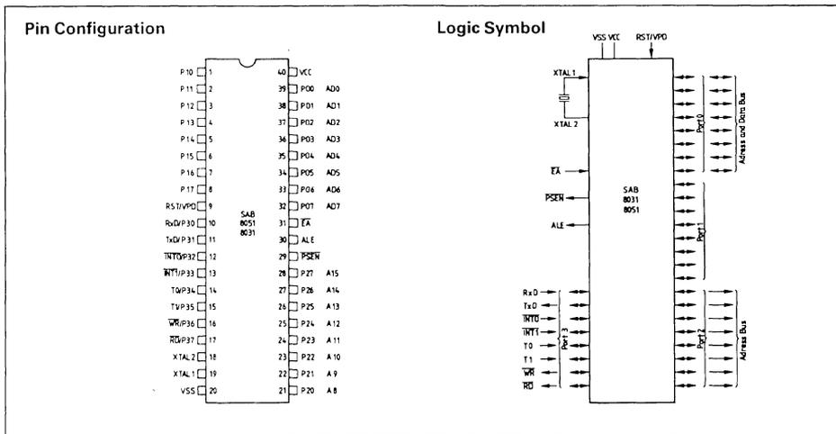
The SAB 8031/8051 for the two extended temperature ranges (Industrial temperature range: -40 to +85°C, Automotive temperature range: -40 to +110°C) is fully compatible with the standard SAB 8031/8051 with respect to architecture, instruction set, and software portability.
