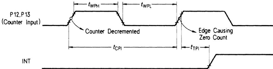
**Loading Timer 5 (or Cascaded Counter/Timer 3 and 5) and Zero-Crossing of Counters (Cascaded Counter/Timer 3 and 5)**
