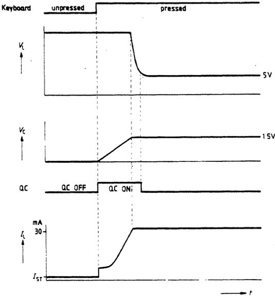
The control circuitry for the quick charging circuit has a hysteresis with the following thresholds:
