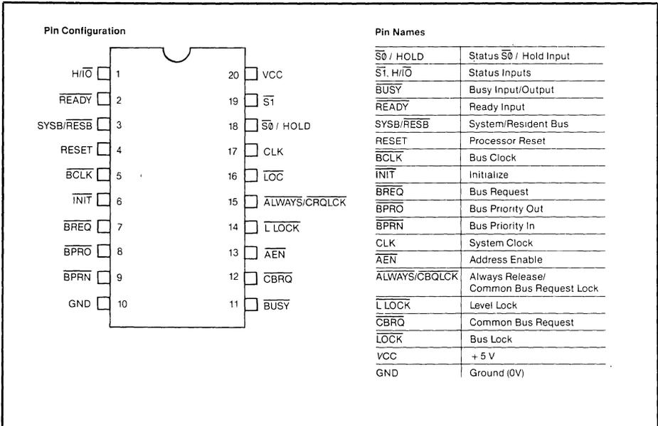
The SAB 82289 Bus Arbiter is a 5-Volt, 20-pin MYMOS component for use in multiple bus master SAB 80286 systems. The SAB 82289 provides a compact solution to system bus arbitration for the SAB 80286 CPU.
