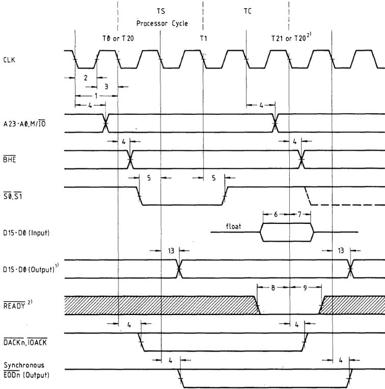
Note 1: D15-D0 floats during Single Cycle Transfer like a Read Cycle.
