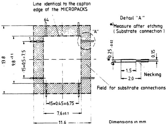
**Note:** Necking of the connection leads is not required in the case of galvanically deposited Sn/Pb and subsequent melting.
