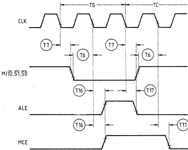
**CENL, CMDLY, DEN Characteristics with MB = 0 and CEN = 1 during Write Cycle**
