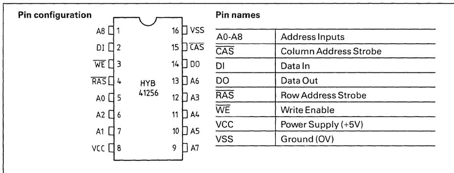
The HYB 41256 is a 262,144 word by 1-bit dynamic Random Access Memory. This 5V-only component is fabricated with Siemens new high performance N-channel silicon gate technology. The use of tantalum polycide provides high speed. A Siemens proprietary chip cover protects the chip against  $\alpha$  radiation.
