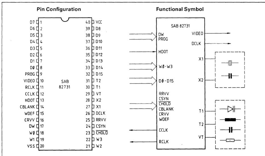
The SAB 82731 is a general purpose video interface, which generates a video signal output for the CRT monitor from parallel character and attribute information coming from the character generator and the CRT controller. The SAB 82731
