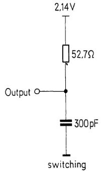
Output Test Load Circuit
