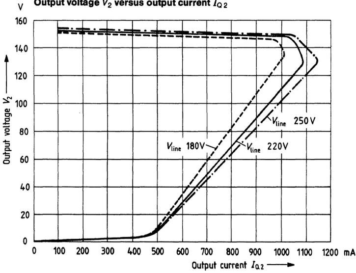
**Output voltage  $V_2$  versus line voltage alterations**
