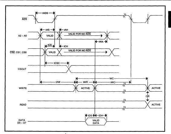
FIGURE 5: Write Cycle Timing
