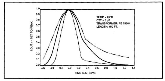
FIGURE 5: Transmitter Pulse Shape for 78P236
