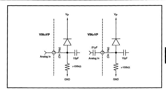
FIGURE 1: Input Coupling
