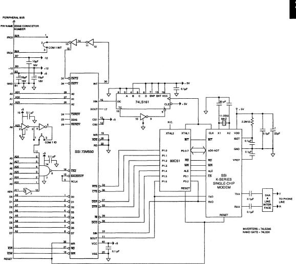
FIGURE 18: Typical Application Showing Modern Interface to Peripheral-Bus via SSI 73M550 UART
