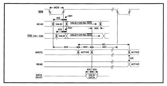
FIGURE 5: Write Cycle Timing
