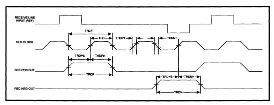
FIGURE 2: Receive Waveforms
