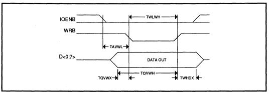
FIGURE 2: LED Write Timing
