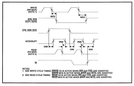
FIGURE 8: Modem Controls Timing
