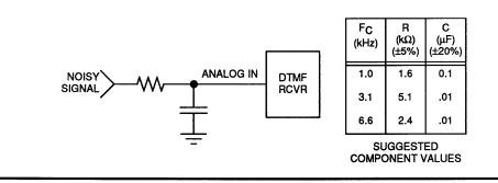
FIGURE 4: Filter for Use in Noisy Environments
