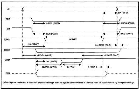
FIGURE 9: I/O Output Timing Specification (WRITE)
