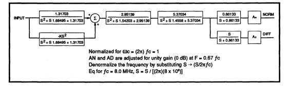
FIGURE 3: 32F8020/8022 Normalized Block Diagram
