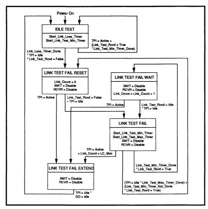
**FIGURE 3: Link Integrity Test Function**
