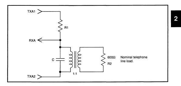
FIGURE 1: TXA Hybrid Loading Analog Interface Hybrid Loading
