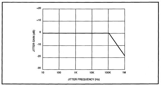
FIGURE 4: 78P236 Jitter Transfer Function Loop Filter BW = 165 kHz
