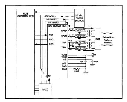
FIGURE 9: Typical SSI 78Q903 Hardware Control Application
