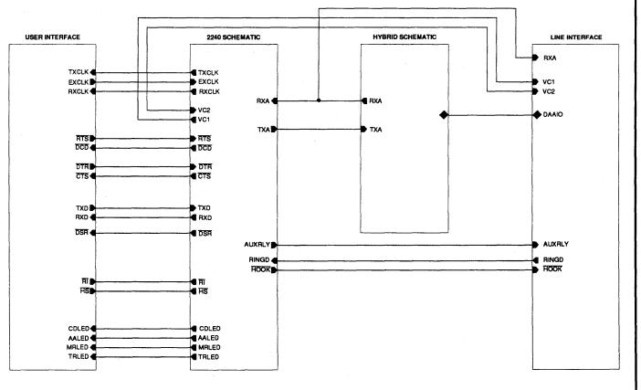
FIGURE 2: SSI 73D2240 Box Modem Block Diagram
