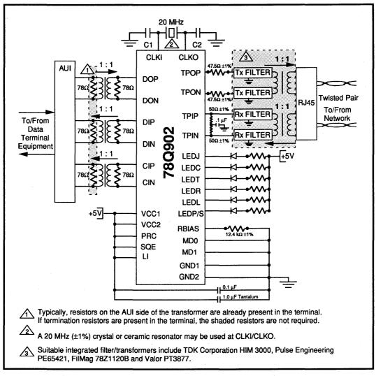
FIGURE 7: SSI 78Q902 External MAU Application Diagram
