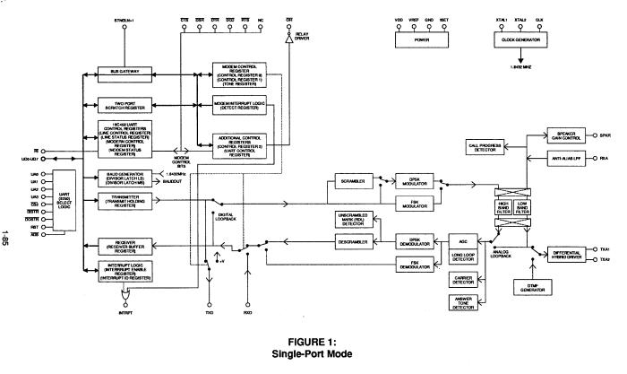
In the single-port mode, the SSI 73K222U is designed to be accessed only by the main CPU using the same parallel bus utilized for data transfer. This mode is enabled when the STNDLN pin is at a logic "1". In the single port mode, internal registers are accessed by the main CPU to configure both the UART section and the
