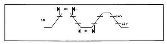
FIGURE 2: External Clock Input\* (4 MHz Maximum)
