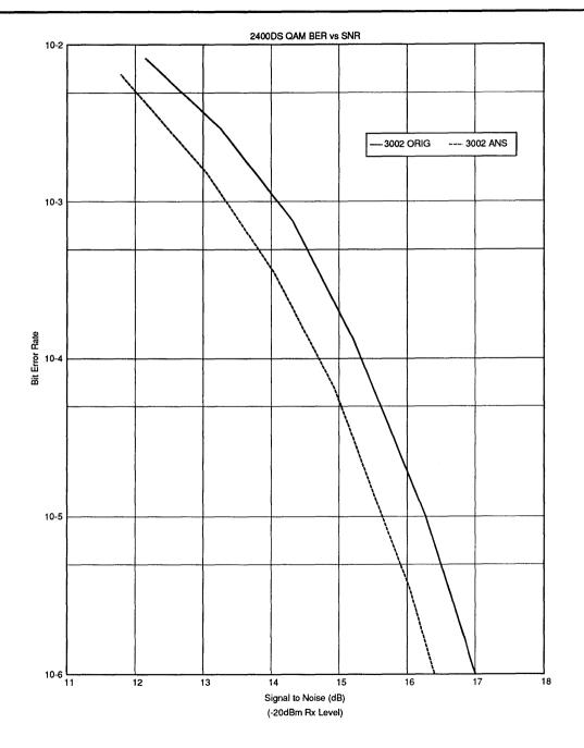
FIGURE 6: QAM and PSK BER vs. SNR with -20dBm Receive Level
