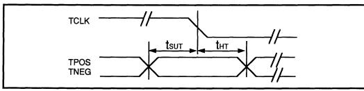
FIGURE 1: 78P300 Transmit Clock Timing Diagram
