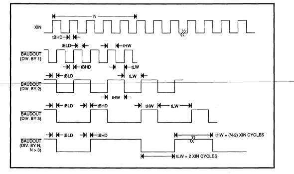
FIGURE 8: BAUDOUT Timing
