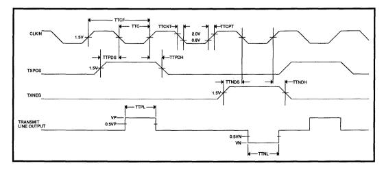
FIGURE 2: Transmit Waveforms
