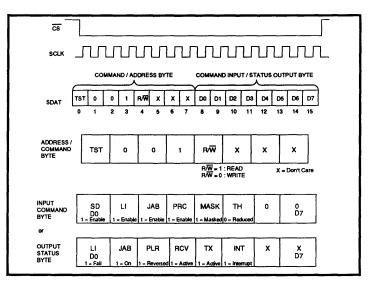
FIGURE 4: Serial Interface Data Structure
