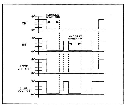
FIGURE 1: Relay Hold and Power Down Timing Diagrams
