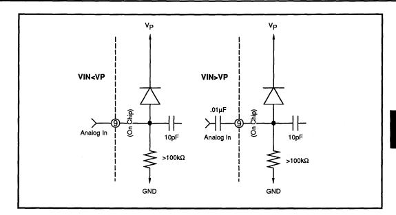
FIGURE 1: Input Coupling
