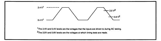
FIGURE 3: AC Test Points\*
