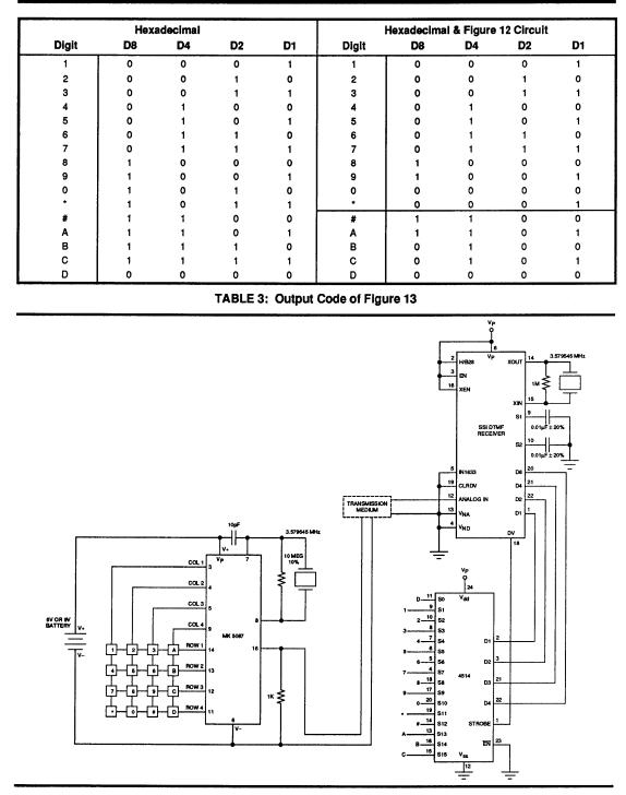
FIGURE 13: 16-Channel Remote Control
