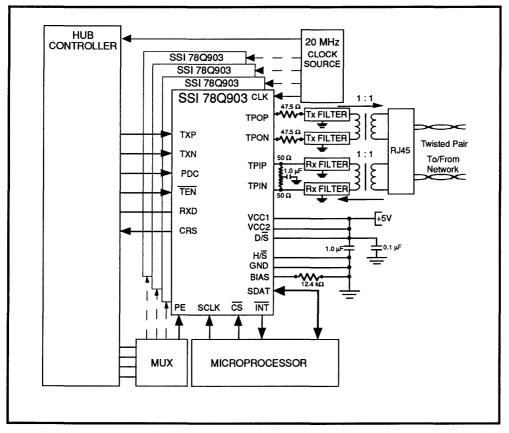
FIGURE 12: Typical SSI 78Q903 Software Control Application
