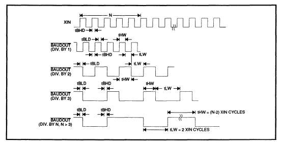
FIGURE 10: BAUDOUT Timing
