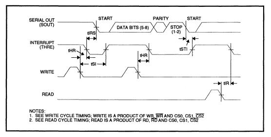
FIGURE 6: Transmitter Timing
