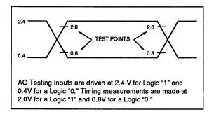
FIGURE 7: AC Testing I/O Waveform
