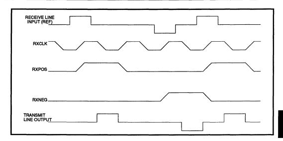
FIGURE 4: Line Loopback Waveforms
