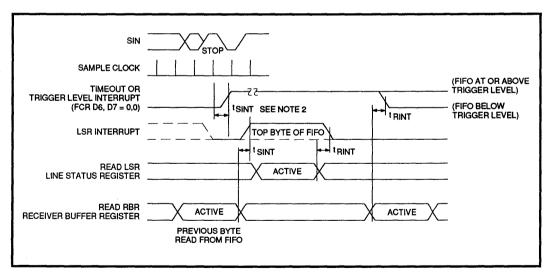
FIGURE 13: RCVR FIFO Bytes Other Than the First Byte (RBR is already set)
