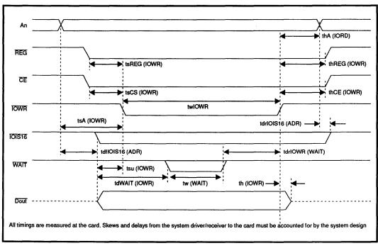
FIGURE 16: I/O Output Timing Specification (WRITE)
