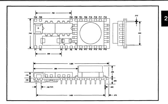
FIGURE 1: Mechanical Diagram
