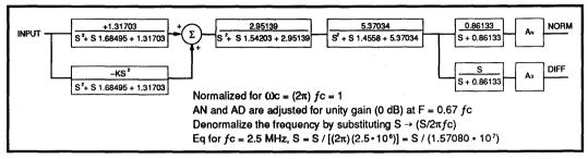
FIGURE 3: 32F8030 Normalized Block Diagram
