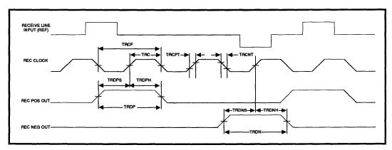
FIGURE 2: Receive Waveforms
