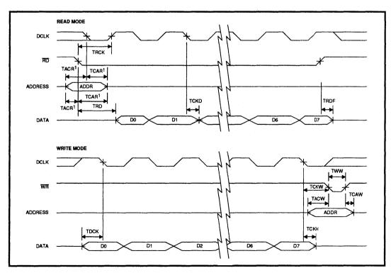
FIGURE 4: Modem Serial Bus Timing
