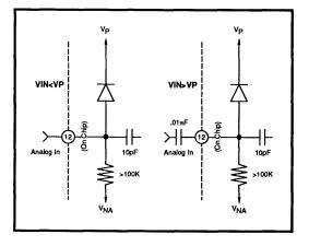
FIGURE 1: Input Coupling
