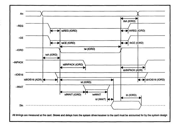
FIGURE 17: I/O Output Timing Specification (READ)
