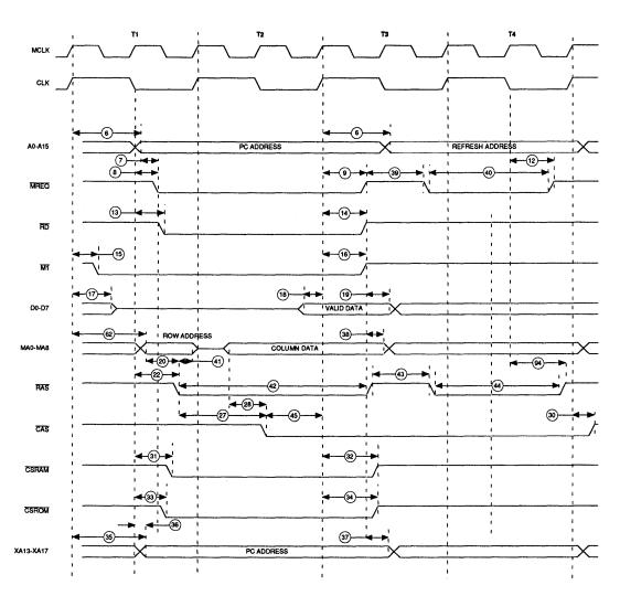
FIGURE 3: Z80 CPU Opcode Fetch Timing – No Wait State
