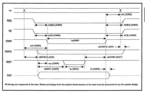
FIGURE 10: I/O Output Timing Specification (WRITE)
