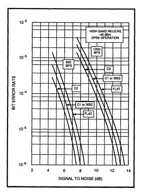
FIGURE 4: SSI 73K222U Typical BER vs. S/N
