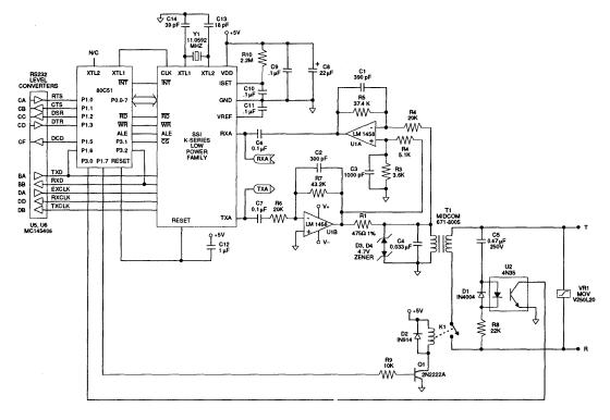
FIGURE 1: Basic Box Modem with Dual-Supply Hybrid
