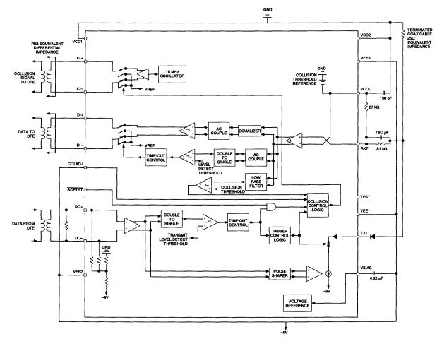
FIGURE 1 : Ethernet Transceiver Circuit Electrical Specification
