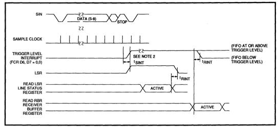
FIGURE 12: RCVR FIFO First Byte (This sets RBR)
