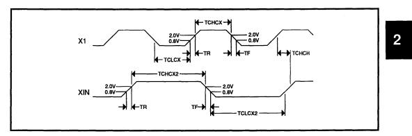
FIGURE 1: Input Clock Timing
