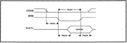
FIGURE 3: Switch Read Timing
