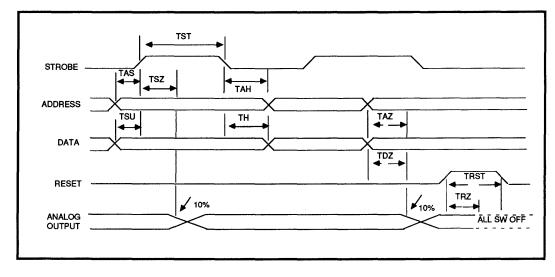
FIGURE 3: Timing Diagram
