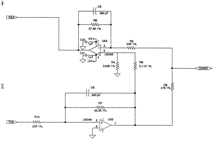
FIGURE 3: SSI 73D2240 Hybrid
