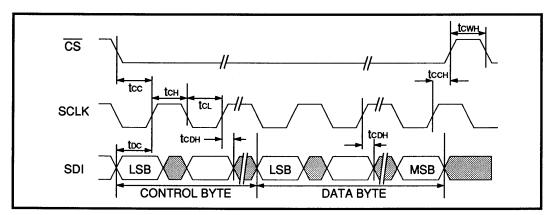
FIGURE 5: SSI 78P300 Serial Data Input Timing Diagram
