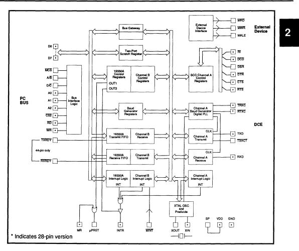
FIGURE 2: Single-Processor Mailbox Mode Block Diagram
