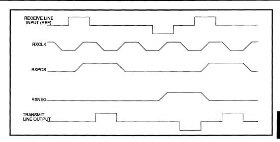
FIGURE 4: Line Loopback Waveforms
