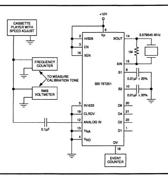
FIGURE 11: Circuit for Receiver Evaluation
