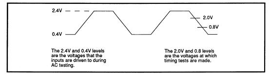
FIGURE 3: AC Test Points\*
