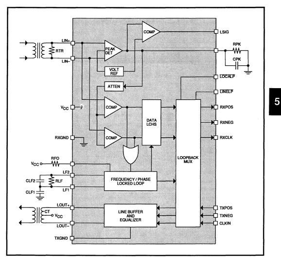
FIGURE 1: SSI 78P234 Functional Diagram
