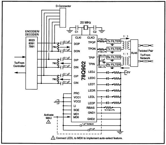
FIGURE 10: SSI 78Q902 Internal MAU Application Diagram
