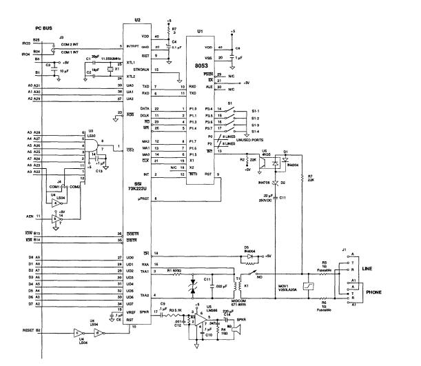
FIGURE 10: 73K22U Typical Integral Application Dual-Port Mode
