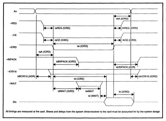
FIGURE 11: I/O Output Timing Specification (READ)
