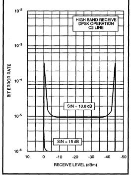
FIGURE 5: SSI 73K222U Typical BER vs. Receive Level
