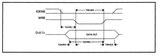
FIGURE 2: LED Write Timing
