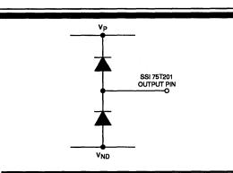
FIGURE 8: SSI 12V DTMF to TTL Level Interface
