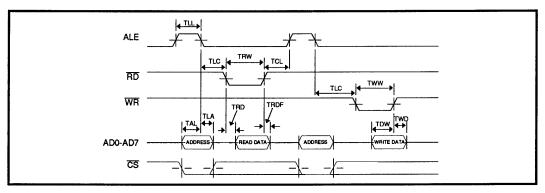
FIGURE 1: Bus Timing Diagram (Parallel Version)
