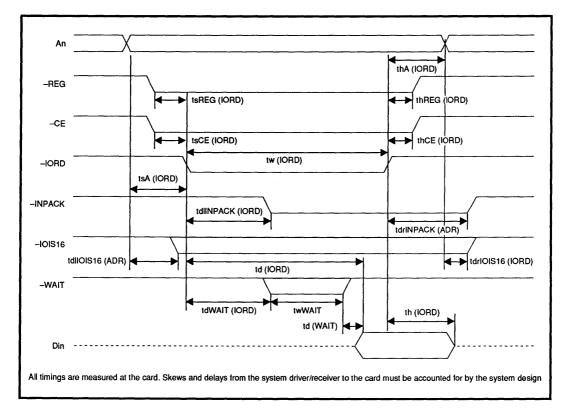
FIGURE 10: I/O Output Timing Specification (READ)
