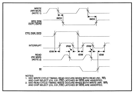
FIGURE 9: Modem Controls Timing
