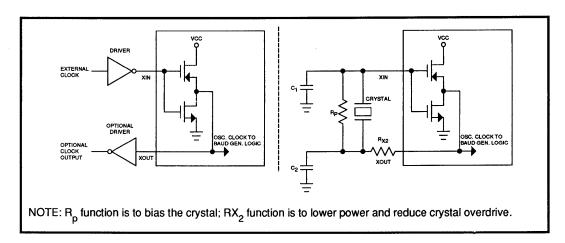
FIGURE 1: Typical Clock Circuits
