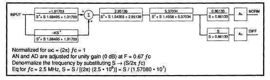
FIGURE 1: Normalized Transfer Function of the SSI 32F8130/8131
