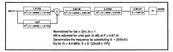
FIGURE 2: 32F8021/8023 Normalized Block Diagram
