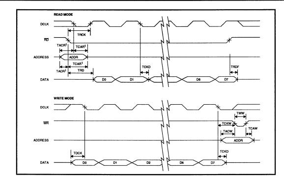
FIGURE 2: Modem Serial Bus Timing
