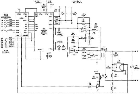
FIGURE 1: Basic Box Modem with Dual-Supply Hybrid
