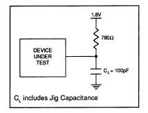
FIGURE 8: Testing Load Circuit
