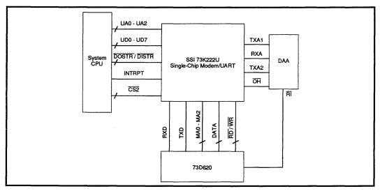
FIGURE 7: Typical Block Diagram for an Internal Modem Utilizing the SSI 73D2180 Chip-Set
