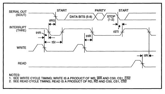
FIGURE 6: Transmitter Timing
