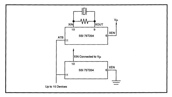
FIGURE 2: Crystal Connections
