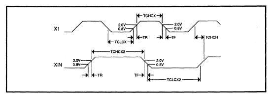
FIGURE 1: Input Clock Timing
