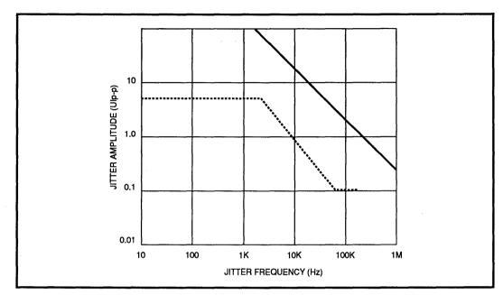
FIGURE 3: Jitter Tolerance for 78P236
