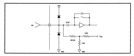
FIGURE 1: VIN Equivalent Input Circuit
