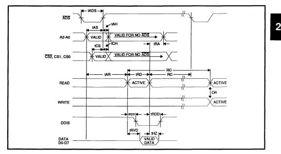
FIGURE 4: Read Cycle Timing
