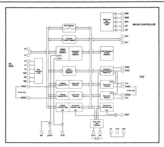
FIGURE 1: Dual-Processor Block Diagram
