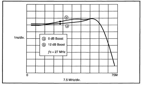
FIGURE 3: 32F8000 Group Delay Response with fc = 27 MHz
