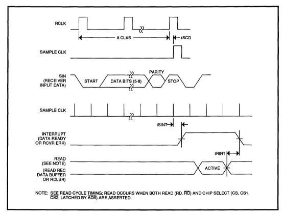
FIGURE 9: Receiver Timing
