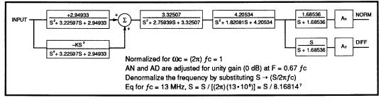
FIGURE 12: 32F8011/8012 Normalized Block Diagram
