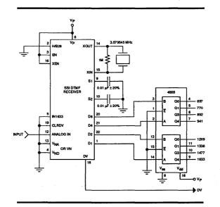
FIGURE 14: Touch-Tone™ to 2-of-8 Output Converter
