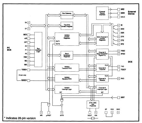
FIGURE 3: Single-Processor Non-Mailbox Mode Block Diagram
