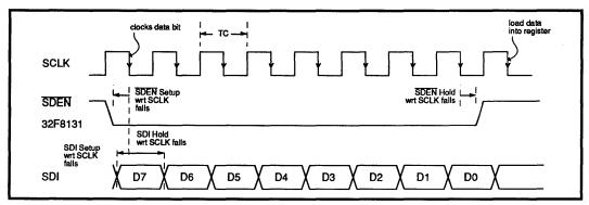
FIGURE 2: Serial Port Timing Relationship
