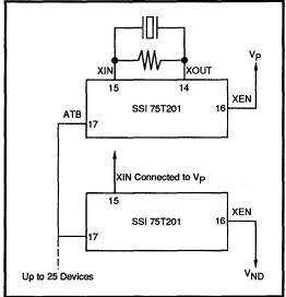
**FIGURE 2: Crystal Connections**
