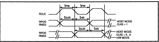
FIGURE 3: 78P300 Receive Clock Timing Diagram
