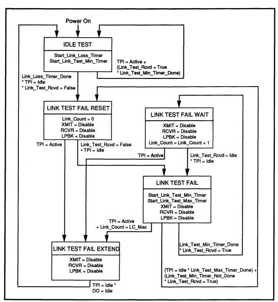
**FIGURE 5: Link Integrity Test Function**
