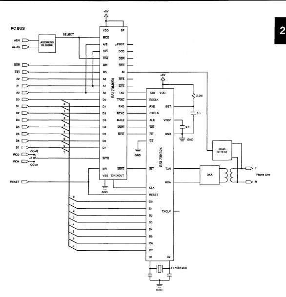
FIGURE 12: Single-Processor Mailbox Mode Application Example
