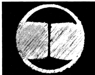
Centerplane cross section of the FLEX-FIT™ compliant pin in a 0.037" diameter finished through-hole.
