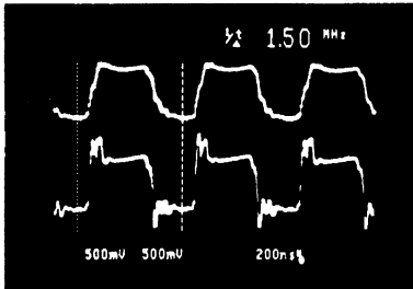
Top Trace Filtered Ip TP'I: .5 v/cm Bottom Trace Unfiltered Ip TP'P: .5 v/cm
