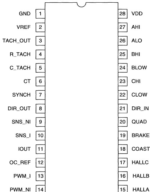
DIL-28, SOIC-28, TSSOP-28 (Top View) N Package, DW Package, PW Package
