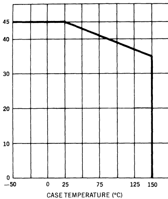
V_{RRM} Rating vs Case Temperature
