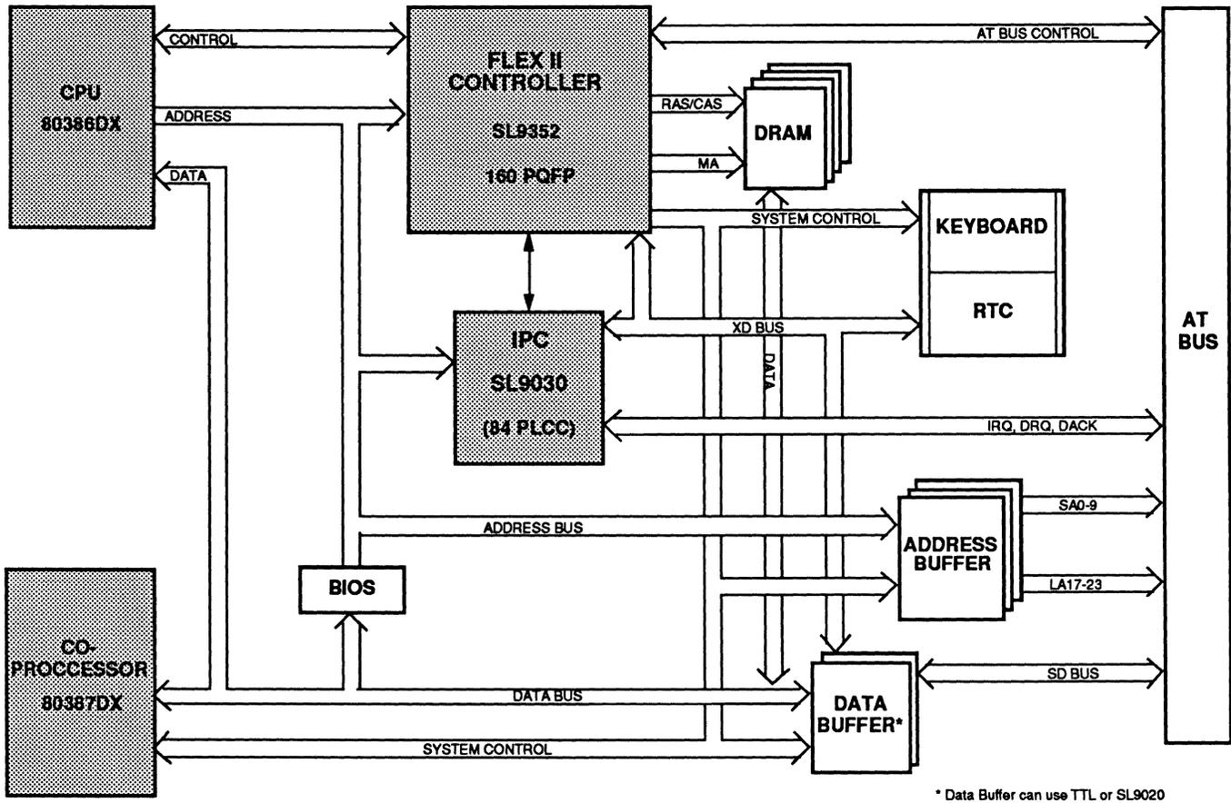
Fig. 1. Block Diagram for 80386DX CPU Board
