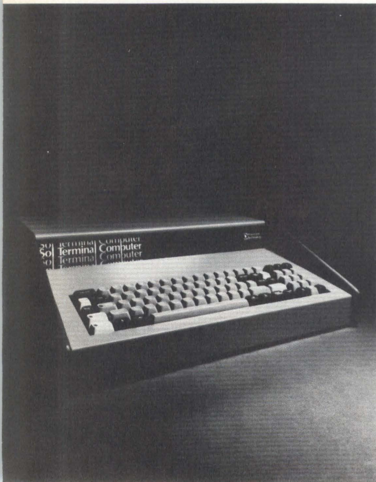
Fig 1 Housed in a typewriter-sized cabinet on which a CRT monitor can sit, Sol-20 contains all circuitry necessary to function either as an intelligent terminal or a stand-alone computer. The system's designers chose to configure it around the "hobbyist," or S-100, bus structure used in several 8080-based computers; Sol is basically the combination of several S-100 peripheral modules with a microprocessor circuit.
