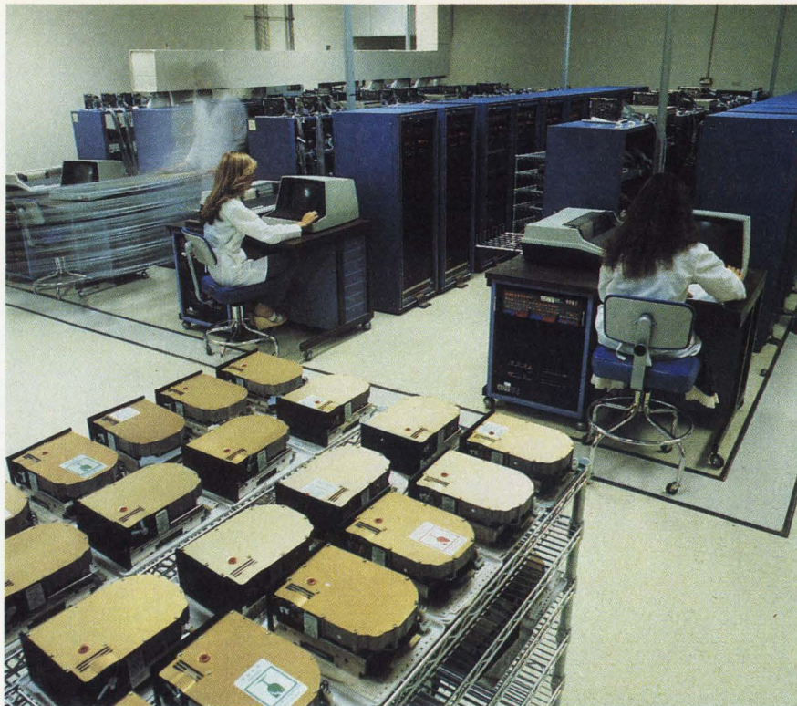
Drives and drive subsystems should be tested on the incoming side of major production phases before integration occurs.
