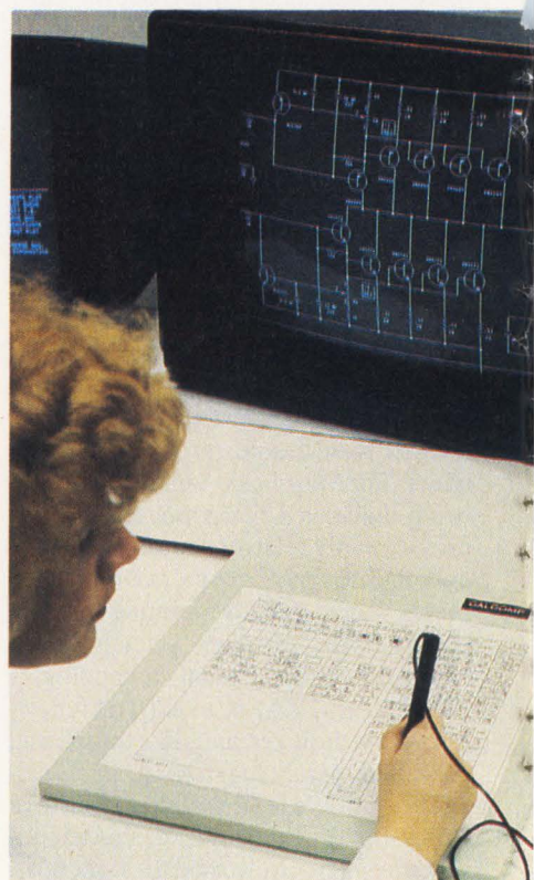
Figure 5: Calcomp's digitizing tablet is used here for input to a CAD system; much of the surface is devoted to menu boxes.
