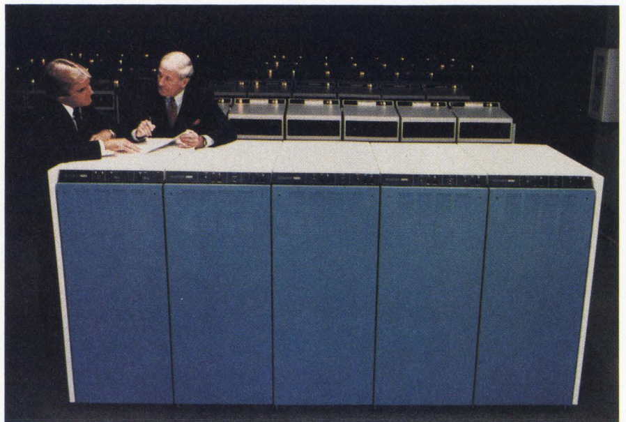
Figure 5: Although functional specs for Memorex's 3680 subsystem are identical to those of IBM's 3380 subsystem, Memorex claims that their drives offer higher performance in high transaction environments.
