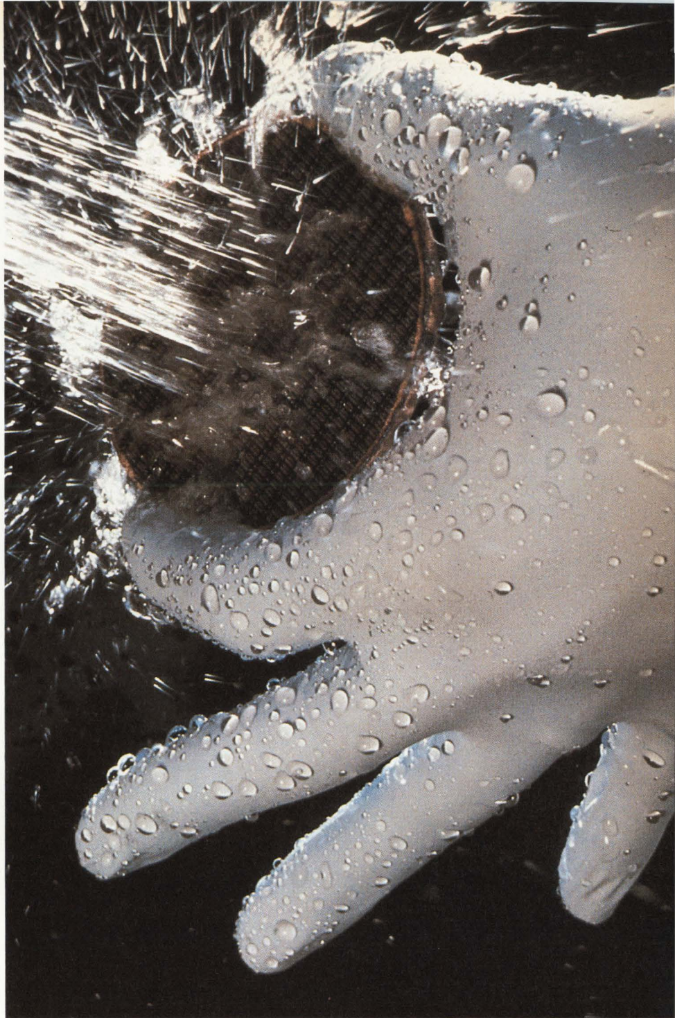
Figure 1: Thin-film heads are batch fabricated in lots of up to 500 on a single silicon wafer (Photo Courtesy Memorex).
