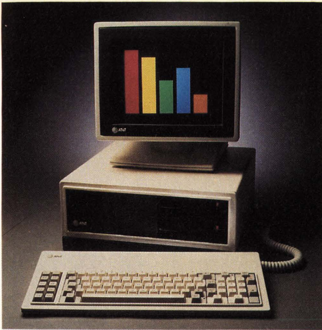
The AT&T PC6300 operates in MS-DOS yet can act as a UNIX dumb terminal.
