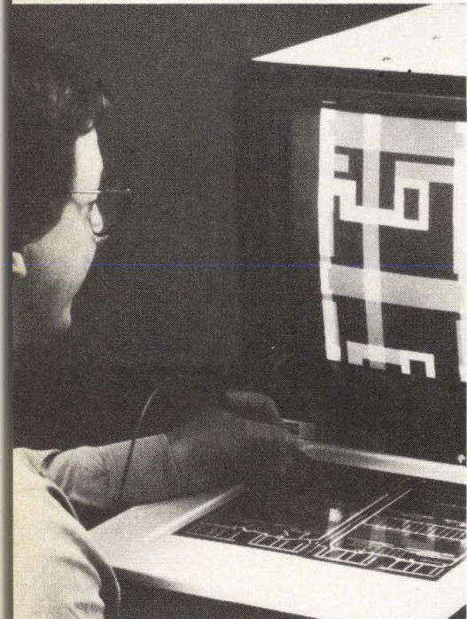
Software support for Peritek's VRH-Q includes a version of GKS, VDI, two levels of graphics subroutines, and an image editor using a mouse.
