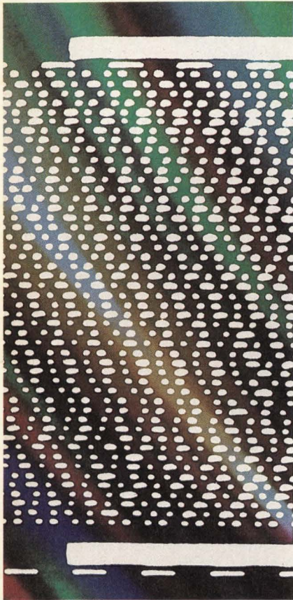
Figure 3: A greatly magnified photo of a recorded band on the STC 7640: the large white areas at the edges are prerecorded band boundaries; the central patterns are user-recorded tracks.
