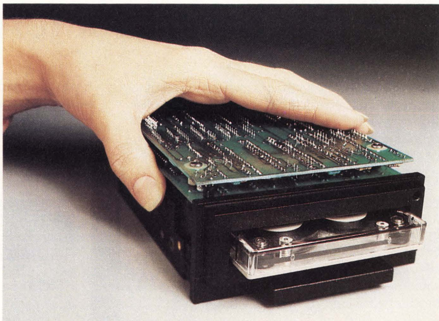
Figure 4: The Irwin Magnetics 210 tape drive fits into a 3.5" footprint and stores 10.38 Mbytes on a single minicartridge tape.
