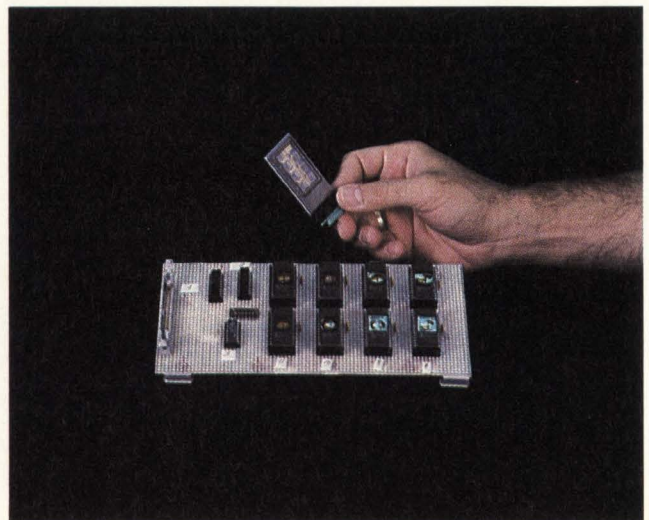
The Medtronic MemoryMod is a small 56 Kbyte, EPROM-based memory cartridge containing seven 27C64 EPROMs plus interface circuitry.
