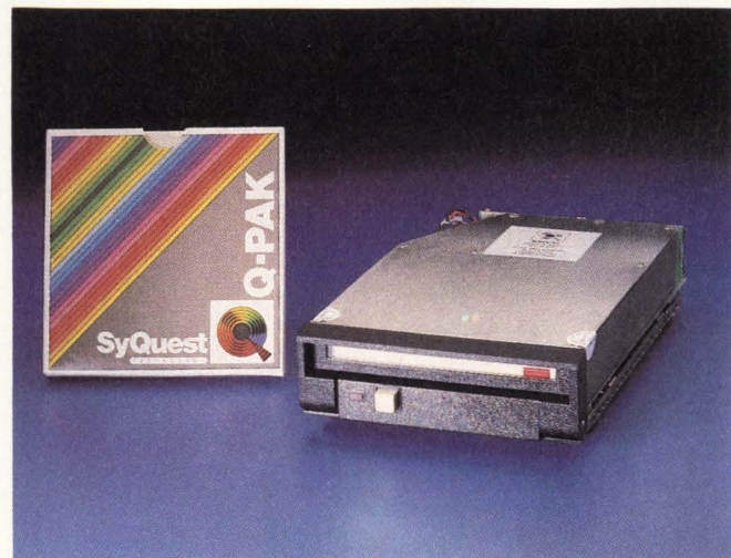
Figure 2: SyQuest's 306RD was the first Winchester to use sub-4" media. The 100mm disk cartridges currently store 5 Mbytes; a 10 Mbyte version is planned.
