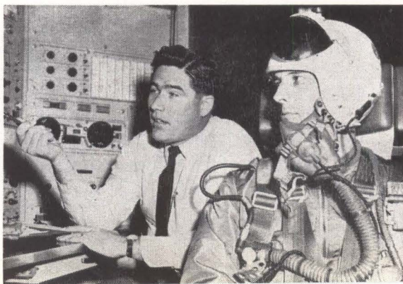
B-58 ecm simulator, already in operation over a year, provides space for instructor not available in airborne training
