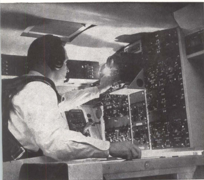
Ecm simulator provides electronic warfare officer all equipment found in the B-52 for detecting and taking action against hostile signal transmission
