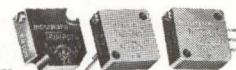
MODEL 3251 Square, high-temperature, Resiston® carbon; 20K to 1 Meg.; 0.25W; Max. oper. temp., 150°C.
