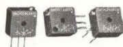
MODEL 3280 Square, micro-miniature, wirewound; 100Ω to 50K; 1.0W; Max. oper. temp., 175°C.
