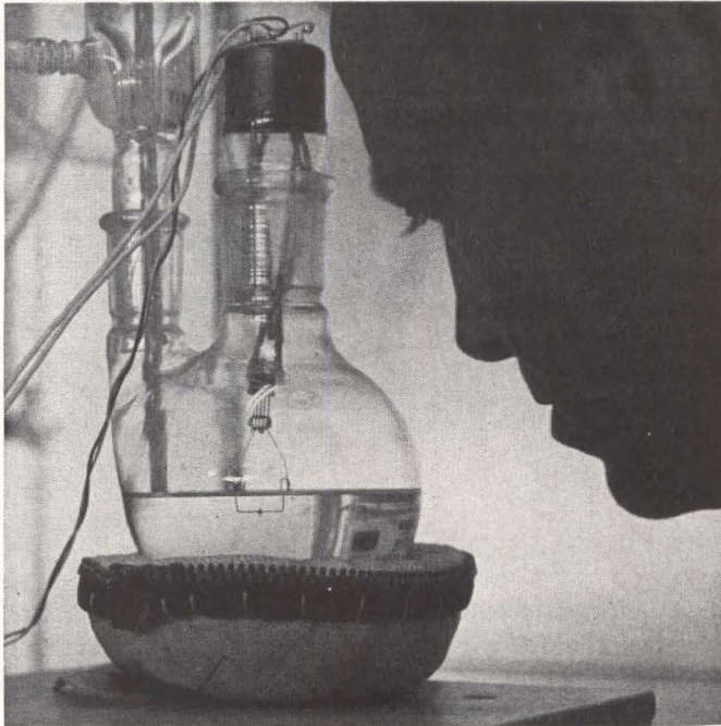
RCA SCIENTIST observes flexode being processed in temperature-controlled silicone oil bath (photo above)
