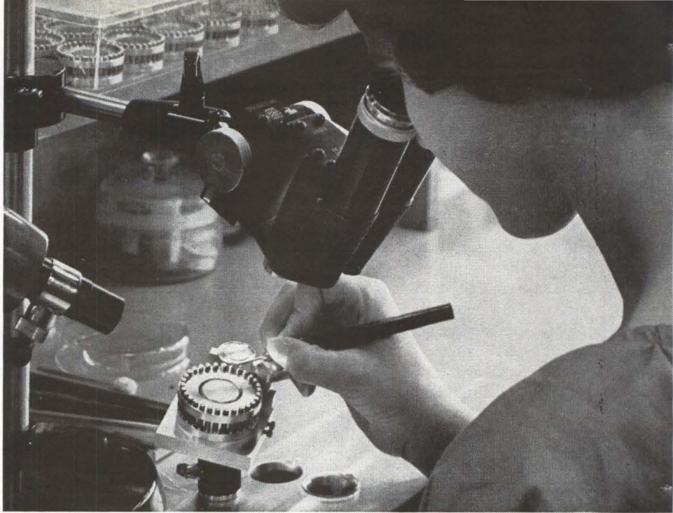
DIODE posts are shown on rotary assembly jigs but pin chip is visible only under microscope
