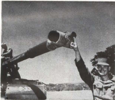
KILLING END of the hit-kill indicator is a photoelectric telescope in the tank's barrel
