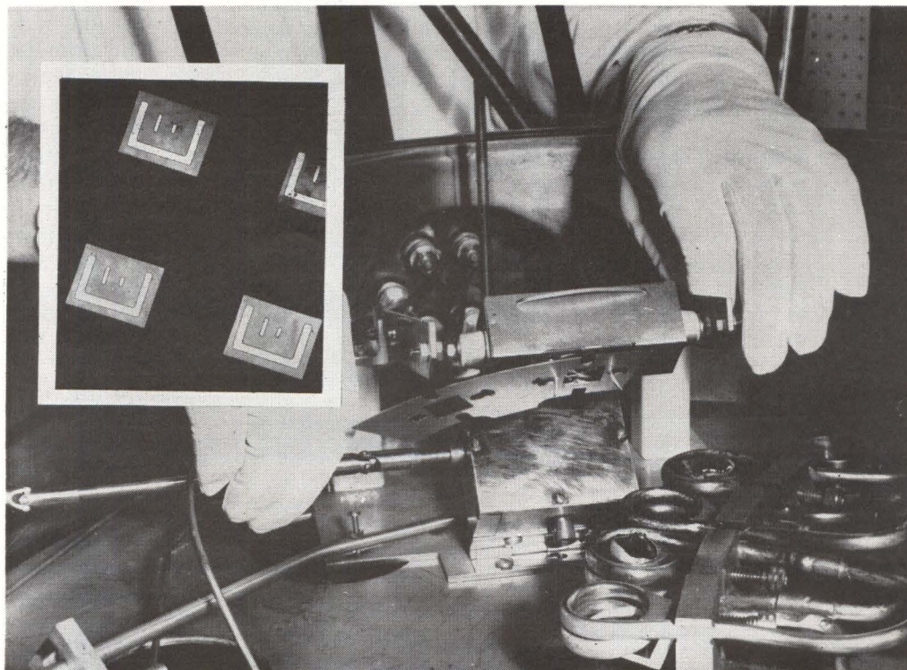
SUBSTRATE HEATER, mask holder and multiple source holder; inset shows vacuum-deposited thin-film transistors with ohmic contacts—Fig. 6
