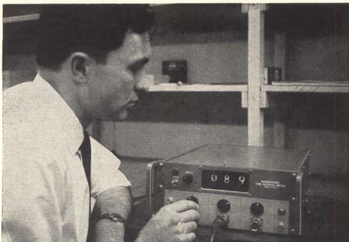
AUTHOR tests a nanosecond time-interval meter that uses the circuits discussed in this article
