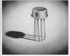
Commercial HLTTL circuits are packaged in this hermeticallywelded TO-5 can with ½" leads.
