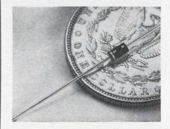
A one-watt zener diode occupies only 0.0016 cubic inches (about the size of a  $\frac{1}{4}$ -watt diode) and is priced below one dollar. The IN4728-64 zener series has a l-w rating at 50°C ambient and is capable of up to 3 w with heat sink. The devices are available in voltages from 3.3 to 100 v in standard tolerances of  $\pm 5\%$  and  $\pm 10\%$ .
