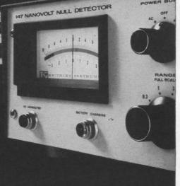
Here's an all-new instrument created especially for sensitive potentiometers and bridges. The 147 electronic null detector gives you resolution of 0.01 microvolt with a 300 ohm source resistance; 0.003 microvolt with 10 ohms. Zero shift of less than 1 x 10<sup>-10</sup> volt per ohm; drift under 25 nanovolts per day; and high line frequency rejection make the 147 a remarkable, universal replacement for even the finest galvanometer systems.
