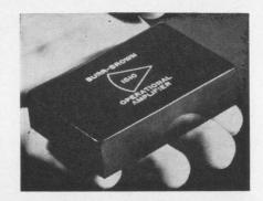
An all-silicon d-c operational amplifier, model 1510, has a bandwidth of 30 Mc with full power response to 1 Mc and a slewing rate of 100 v per  $\mu$ sec. Output is  $\pm 10$  v at 30 ma with only 12 ma quiescent drain from the nominal  $\pm 15$  v external power supply. D-c gain of 30,000 and stability of  $\pm 10 \ \mu v/^{\circ}C$  and  $\pm 0.5 \ na/^{\circ}C$  are typical.
