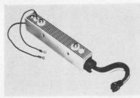
A full-kilowatt, X-band traveling wave tube, the QKW1132, has a unifilar, helix-type wave propagating structure and employs an integral permanent magnet. The rated 1-kw output with an average gain of 40 db applies over the tube's frequency range of 7 to 11 Gc. The conduction-cooled twt is designed for pulse operation with a maximum duty cycle of 0.01. Output vswr is 2:1.
