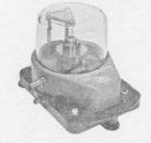
CEC's 6-201 Primary Pressure Standard has long been accepted as the finest of all pneumatic piston gages.
