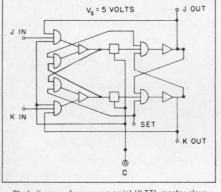
Block diagram of new commercial HLTTL master-slave flip-flop.
