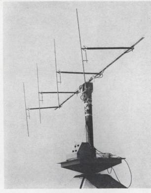
Steerable-beam array made up of four antennafier elements spaced a half-wavelength apart. Beam position could be controlled by a series of four ganged potentiometers.
