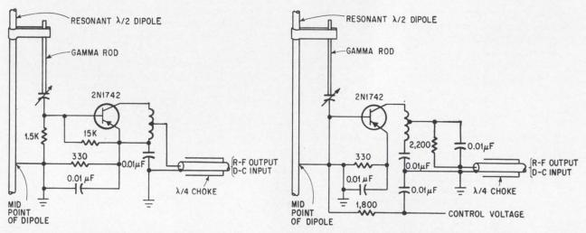
Transistorized dipole antennafiers. Fixed gain is shown at left; controllable gain by external voltage, at right.
