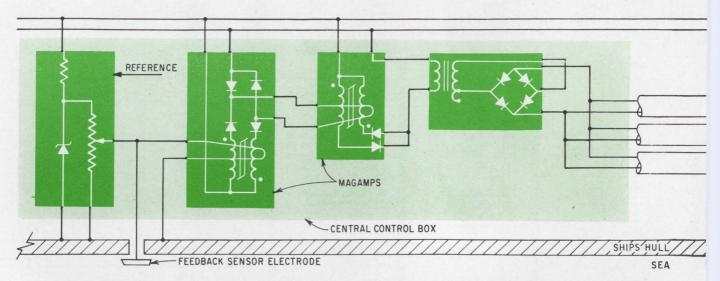
Anticorrosion system laid out partly as a pictorial representation of how the equipment would be installed on a ship and partly as the classic feedback control system diagram. The steel hull of the ship is the system signal and power ground. The reference voltage at the left commands the amount of voltage difference to be impressed on the hull. The
