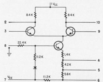
Monolithic differential ampilier MC1525 uses this basic circuit. Additional resistors have been included, which the customer may use or omit depending on the current level of operation. Numbers on the circuit identify leads.
