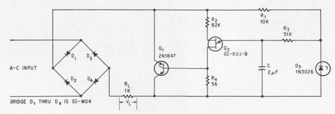
Firing angle of the silicon controlled rectifier varies with amplitude of the input a-c voltage; this variation maintains constant average voltage across load R<sub>L</sub>. Load voltage can be adjusted by changing the value of R<sub>1</sub>.
