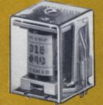
Tab terminals for PCB mounting Type LB Relay has tinned nickel silver terminals for direct PCB mounting. Volume: 1.33 cubic inches. Maximum mounted height, 1.24 inches. Relay shown actual size.
