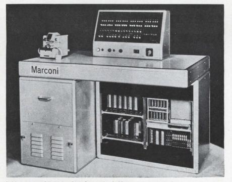
Achievement of British microelectronics is Marconi Co.'s desk-size Myriad computer measuring 6 by 3 by 2<sup>1</sup>/<sub>2</sub> feet. It has 4,096-word capacity, can add and subtract in 2.5 microseconds and multiply in 10 microseconds. Maximum time before failure is said to be 30,000 hours, compared with 3,500 hours for most conventional models. First model has been sold to Royal Radar Establishment at Malvern.
