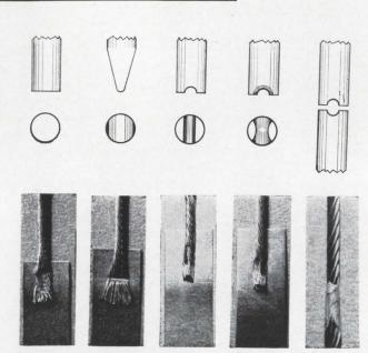
Five shapes for electrodes and the welds they make. Left to right: conventional flat electrode, chisel-shaped electrode, grooved electrode, saddle electrode and pair of grooved electrodes used for splicing two stranded wires by forging ends of the wires together.
