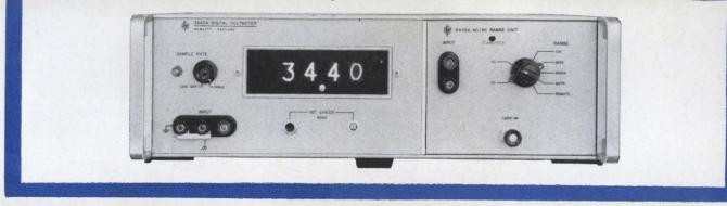
Now your Hewlett-Packard solid-state 3440A DVM lets you measure ac (50 cps to 100 kc) or dc signals 10 to 1000 volts full scale. Just connect directly to the input terminals of the 3445A, select manual range or automatic ranging—or program range remotely. Signal common may be connected up to 500 v dc above ground. Permanent test records are available on all functions, including polarity, decimal, function and overload, with accessory J74-562A Printer for a 1224 code (J76-562A for a 1248 code).
