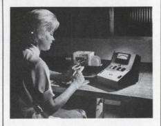
A complete weld station now available offers push-button selection of both energy and force settings. Designed for high-speed production welding applications, this modular automatic weld station (MAWS) provides instant selection of six highly repeatable weld conditions. The result is fewer decisions for the operator, reduced fatigue, fewer rejects.
