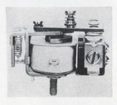
A medium power relay, the 25PD rated at 25 amps, is said to offer greater reliability and better performance than other competitively priced relays. The manufacturer claims extremely long mechanical life for the relay; electrical life is dependent on load characteristics. An important advantage is lower pull-in voltages (d-c: 75% of nominal voltage; a-c: 76% of nominal voltage).
