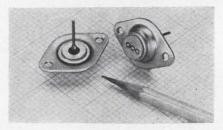
A series of diffused-junction, 25amp silicon power diodes are mounted in heat sinks identical to the TO-3 case configuration, yet are competitive in price to unmounted press-fit diodes. Designated P50S through P400S, the diodes are rated 25 amps output at 100°C in piv ratings from 50 to 400 v, and are available in forward or reverse polarity.
