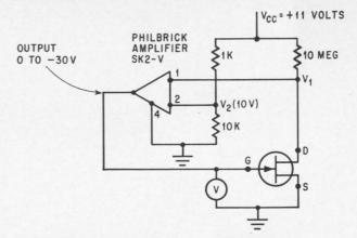
FET drain-to-source pinchoff voltage is obtained indirectly, by measuring gate-to-source voltage that causes  $I_{\rm D}=0.1$  microamperes.
