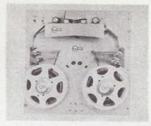
A high-speed photocell punched tape reader and matching tape spooler is announced. The units are designed as input devices for numerical control systems, digital computers, automatic drafting machines, automatic circuit evaluators, or other systems requiring reliable, high-speed punched tape reading.
