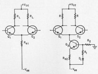
**Tenfold increase in impedance** results from substituting transistor (diagram at right) for emitter resistor in diagram at left. Limitations of monolithic circuits restrict size of resistor R<sub>e1</sub> to about 20,000 ohms. Transistor increases impedance to 200,000 ohms or more. Only 1% of area needed by 200,000 ohm resistor is used.
