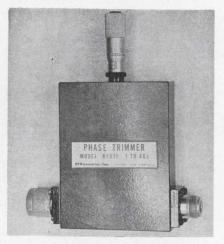
A noise-free coaxial phase trimmer, model Rf311 has no sliding metalto-metal contacts. It is used as a coaxial line stretcher where a fine control of phase of a microwave signal is required. Control is manual with a micrometer drive for ease of calibration and assurance of resettability. A lock nut on the micrometer prevents accidental change of setting.
