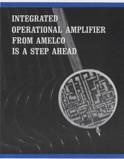
**NOW** you can obtain the advantages of high reliability and small size inherent in monolithic diffused integrated circuits **and still get an output voltage swing of 20 volts.** This and other important parameter limits given below are all available — from stock — in the A13-251. The budget saving price is \$44.50 for small quantities and \$35.50 for 100 or more.
