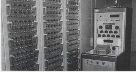
In order to accommodate the 10,000-hour failure-rate level determination load life test (shown above) as well as the other special tests required by MIL-R-39008, Speer recently added 28,000 square feet of quality control and inspection facilities to its Bradford, Pennsylvania, resistor plant.
