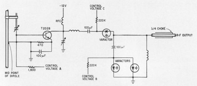
Dipole antennafier with phase shifter is one element of steerable-beam array.
