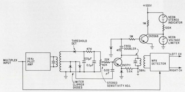
Multiplex module is prevented from operating when multiplex signal is below an acceptable power level. In this case, f-m reception is monaural.
