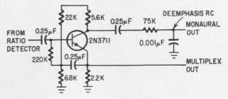
Final stage of i-f amplifier module has two outputs to allow independent operation of monaural f-m.
