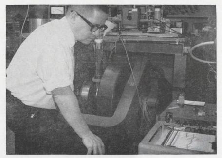
**Scientist watches readout** of electron-spin resonancy device (to his left) that is testing a sample of human tissue for cancer. The device detects malignancy because of the peculiar way the diseased tissue reacts in an intensive magnetic field.
