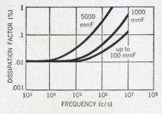
Low dissipation factor (usually even lower than for mica capacitors) is provided by Styroflex capacitors... making them specially suitable for filter circuits.
