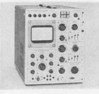
Type 549 oscilloscope combines the features of the 545B with the added versatility of storage capability. It has what is believed to be the fastest-writing bistable storage crt. The 6-cm by 10-cm display area is divided into two 3-cm by 10-cm independently controlled targets for split-screen applications, plus a nonstoring "locate" zone at the left and a "run-over" storage area at the right.
