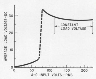
**Regulation curve** shows that the average load voltage is constant at about 30 volts, as the input a-c voltage varies from 100 to 200 volts rms.
