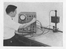
Frequency-response curves and return loss curves, calibrated directly in decibels, are traced out continuously during microwave sweptfrequency tests by a plug-in model 1416A for the model 140A oscilloscope.
