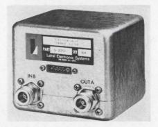
A series of tracked/isolated YIG electronically tunable microwave filters are said to offer lower insertion loss, improved tracking characteristics, broader bandpass and lighter weight than those introduced by the manufacturer a year ago. The 2200 series units provide two r-f filter sections within the same magnetic tuning structure—a concept that enables the units to be used in advanced electronic equipment, such as doppler radars, ecm/ eccm systems and frequency agility radars.
