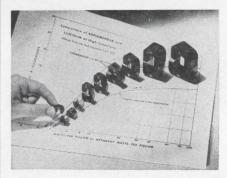
A line of C-cores now on the market is made of Supermendur, a space age alloy of 2% vanadium, 49% iron and 49% cobalt, that permits practical savings in volume from 15% to 40% and weight from 10% to 30%. Performance capability is comparable to C-cores that are  $\frac{1}{3}$  larger.
