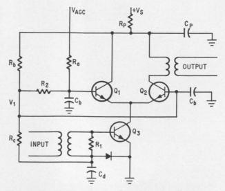
This circuit maintains constant impedance levels while shunting the signal into either the output transistor or the non-output side of a differential pair. This minimizes problem of bandwidth variation and interstage detuning with automatic gain control in tuned i-f cascade amplifiers. The AGC, applied as a differential d-c voltage between the bases, determines the amount of signal shunted to each side. Stage gain is 20 db at 60 Mc.
