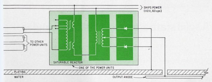
magnetic amplifier chain raises the power level to the several kilovolt-ampere level needed to drive the output anodes. These anodes supply the ion-current flow in the sea water that interacts with the ship's hull to change its voltage several hundred millivolts. The feedback sensor electrode measures the actual hull-seawater voltage differential.
