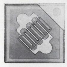
Until six months ago, the highest frequency at which a field-effect transistor could operate as an amplifier was 300 megacycles per second. To overcome this 300-Mc barrier, Texas Instruments Incorporated engineers investigated several geometries which could produce higher transconductanceto-capacitance ratios. They found that interdigitated geometry, in conjunction with epitaxially deposited junction areas, met the requirements, and combined these two techniques in the 2N3823.
