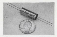
Model 3D2-10 lumped constant delay line features a hermetically sealed case. Delay time is 200 nsec  $\pm 3\%$ ; impedance, 100 ohms; temperature range,  $-55^{\circ}$  to  $+105^{\circ}$ C; size, 1 inch long by 0.4 inch o-d. Units have glass to metal terminals, nickel plated case, and meet MIL-D-23859. Price is \$13 in small quantities; delivery, 2 weeks. Data Delay Devices, 62 Railroad Ave., Paterson, N.J., 07501. [404]
