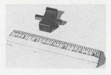
These fixed attenuator pads cover EIA waveguide sizes WR28 to WR90. The units, spanning the frequency range 8.5 to 37 Gc, have a maximum vswr in most cases of 1.20 or less and find wide application in test bench set-ups and local oscillator portions of waveguide subassemblies due to their compact size and excellent electrical characteristics.
