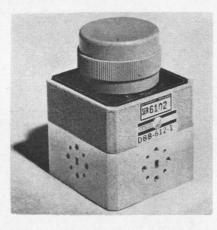
A B size (50 to 75 Gc) manually operated waveguide switch, model DBB-612/614-1, offers maximum insertion loss of 0.2 db, typical isolation of 65 db, and typical vswr of 1. Total weight of the switch is 12 oz. It is 2 in. square by  $2\frac{15}{16}$  in. high. Both single-pole double-throw and double-pole double-throw configurations are available.
