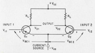
**Typical differential amplifier circuit.** Input signals are  $V_{11}$  and  $V_{12}$ ; differential output voltage is  $(V_{01}-V_{02})$ .
