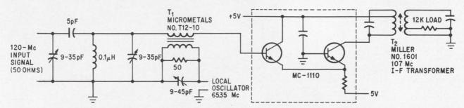
Differential amplifier integrated circuit used as harmonic mixer. Local oscillator operates at half of the intended mixing frequency, and odd-order harmonics are canceled in the mixer. Wide separation of oscillator and signal frequencies allows more effective rejection of spurious responses. A conversion gain of 33 db from 120 Mc to 10.7 Mc can be attained with available integrated circuits such as MC-1110. Low-frequency crystals can reduce cost in vhf range.
