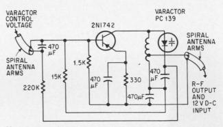
Varactor-tuned transistor amplifier is built into the tip of a conical spiral antenna. Antenna arms are formed by the external sheath of a coaxial cable.
