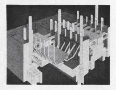
As many as 20 flatpacks and 14 layers of interconnect wiring can be packaged in 1.2 cubic inches with the Omni-Comb interconnection system. The system consists of five basic off-the-shelf parts that can be combined in a prototype or production stage to produce analog or digital subassemblies in practically infinite variety.
