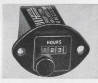
Instantaneous zero reset by a convenient face-mounted push button is featured by these microminiature elapsed time indicators. The units offer a three-digit display of hours or hours and tenths. They may also be allowed to recycle automatically and thus count beyond 999, or 99.9, as applicable, if desired. The indicators are synchronous motor driven.
