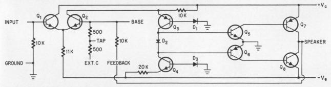
**One-watt integrated-circuit audio amplifier** has negative d-c and a-c feedback applied to one side of a differential input stage; signal is applied to the other side. With balanced power supplies, the output d-c voltage remains at ground potential, allowing a loudspeaker to be driven directly without a large d-c decoupling capacitor. The integrated circuit is the MC1524, a commercially available multi-chip device.
