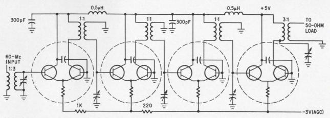
60-Mc intermediate-frequency f-m limiter formed by four differential-amplifier integrated circuits. The circuit provides 80-db power gain at 60 Mc, with a 6-Mc bandwidth and a 6-db noise figure. With microminiature toroid transformers and compact trimmer capacitors, the entire i-f strip package is about 0.2 by 1.2 by 2.3 inches.
