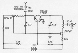
Amplifier in experimental 420-Mc slot antennafier has 10 db gain and noise figure of 7.8 db; bandwidth is 100 Mc.
