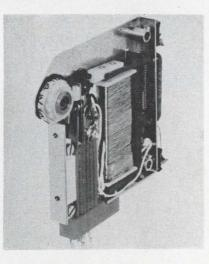
Model WR-25 single decade printer incorporates an escape mechanism that permits the counter to be zeroed with only one 400-msec pulse. Presently, all similarly designed printers must provide a series of pulses in order to be zeroed.
