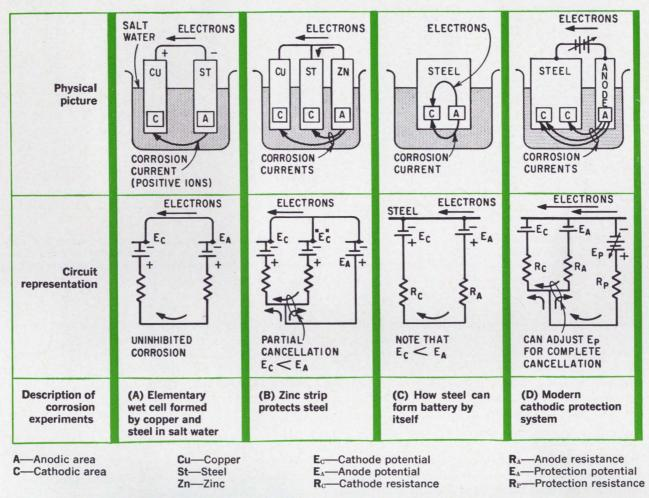
The corrosion of a ship's hull occurs for the same reason that the anode of an electrochemical cell is eaten away. If a strip of steel and a strip of copper are placed in an electrolyte and electrically connected, as in sketch A of the illustration above, a current will flow because the two metals are of different potential. Steel is negative with respect to copper, but the steel will become the anode because it is the source of the positive current through the cell.
