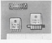
Polar Relay Type 21 Fujitsu Polar Relay Type 21 ts a hermetically sealed, highly sensitive subminiature polar relay with high speed and long service life. The size of this Type 21 is only 1/10th as large as the conventional polar relays. It has extremely efficient magnetic circuits, high stability against external magnetic
