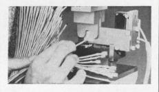
This triggering device is reported to speed up the application of terminals to wires by 40% to 65%. Applicable to wires as fine as 26 gage stranded, the terminal trip device uses a mechanically actuated sensing plate to energize a highly sensitive switch. The switch, in turn, cycles ordinary terminal installation tooling.
