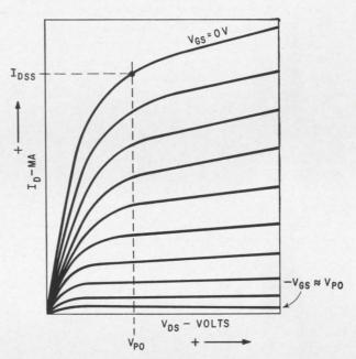
Typical FET drain characteristics.  $V_{\rm PO}$  is drain voltage that causes little or no change in  $I_{\rm D}$  when  $V_{\rm Gs}=O_v.$
