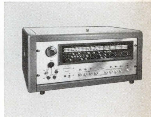
Sequence programmer uses AMP's Matrix Pinboard with interchangeable program templates.
