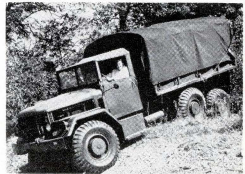
Electrically driven truck, developed for the Army by Lear Siegler, Inc., uses a frequency-control device to regulate speed of electric motors. Each of the six wheels has its own motor. The 2½-ton truck is said to consume about 20% less fuel than a comparable truck driven directly by a gasoline engine.
