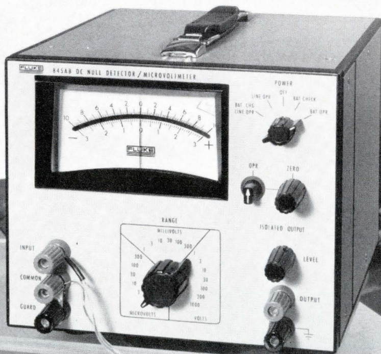
New Fluke Model 845AB checking out Rosa type resistors in oil bath.
