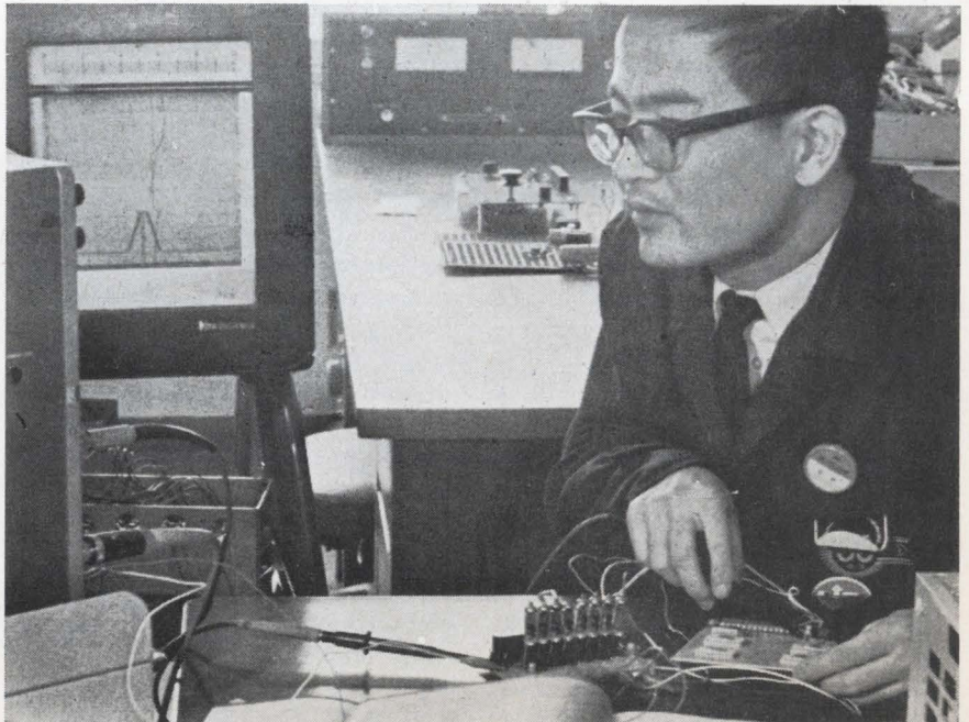
Building blocks. Hayakawa's LSI calculator carries all its logic circuits and display circuits on two small printed circuit boards. Larger board takes care of the four MOS LSI packages plus an IC clock and an IC display driver. Smaller board has the display tubes and their hybrid drive packages. Undersides of boards have only wiring on them.
