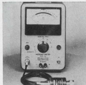
Microwattmeter model 41A covers a range of 200 khz to 12.4 Ghz. It features a single power head measuring down to -60 dbm with dynamic range of 70 db. The system requires no zeroing, except for fractional microwatt measurements, and has an over-all accuracy of \pm 0.5 db. The power head offers overload protection to 300 mw c-w. Boonton Electronics Corp., Parsippany, N. J. [367]
