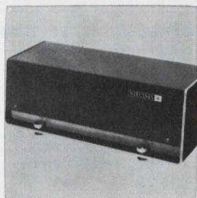
Advanced Nd:YAG laser model 610 is for use where a high power, c-w, 1.06 micrometer source is required. External mirrors and a continuously adjustable output are featured. Unit emits more than 1 w of power in the TEM 00 mode and over 5 w in multitransverse mode operation. Optical length of the laser cavity is 38 cm. Sylvania Electronic Systems, Box 188, Mountain View, Calif. [382]
