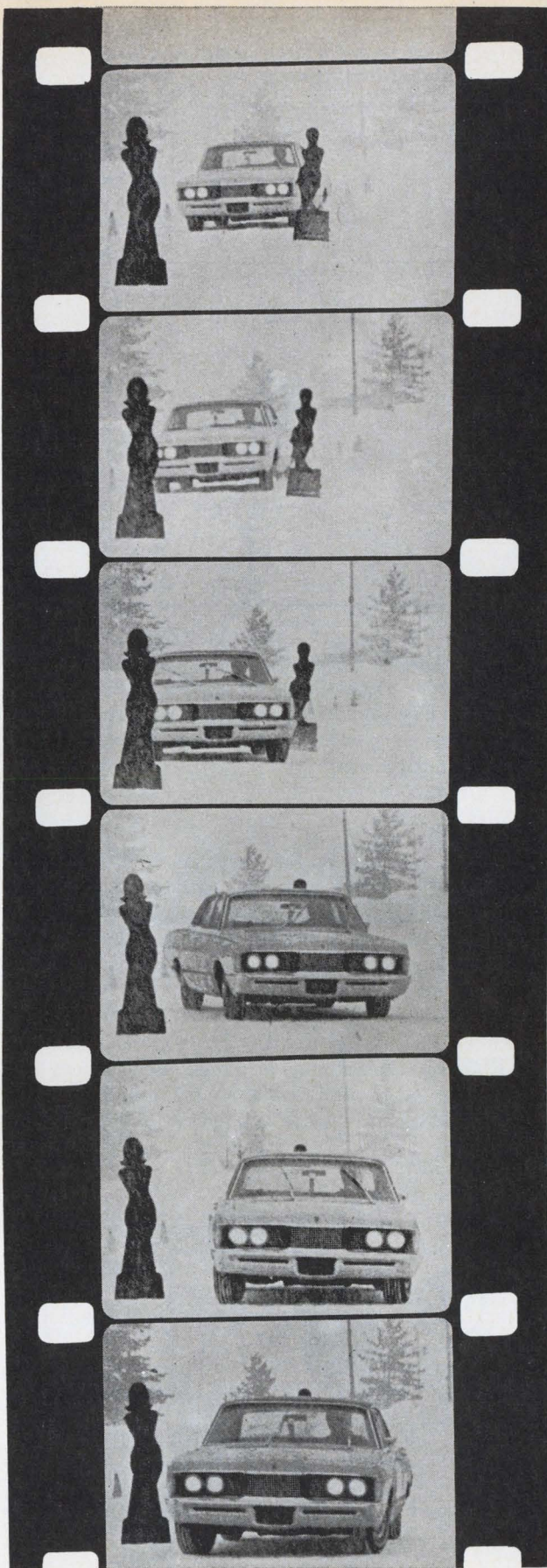
Slalom. These frames from a film made by Bendix show a car equipped with the company's four-wheel adaptive braking system being put through an obstacle course on a slippery proving ground in Bemidji, Minn.
