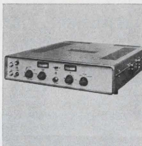
The wide d-c error-voltage swing provided by models 243-T and 247 sweep-lock synchronizers offers a practical means for phase-locking two microwave or r-f sweep oscillators 30 Mhz apart. Each synchronizer can deliver an error-voltage excursion of up to 40 v, enough to drive most sweep oscillators over their entire spectrum. Sage Laboratories Inc., 3 Huron Dr., Natick, Mass. [403]
