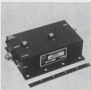
Transistor power amplifier S230 functions as a transmitter in microwave communications systems. When factory tuned to any frequency between 1.85 and 2 Ghz, a power output of 2 w can be obtained at room temperature. For field tunable applications a power output of 1.6 w can be obtained over the 1.85 to 1.99 Ghz range. RCA Electronic Components, Harrison, N. J. [405]
