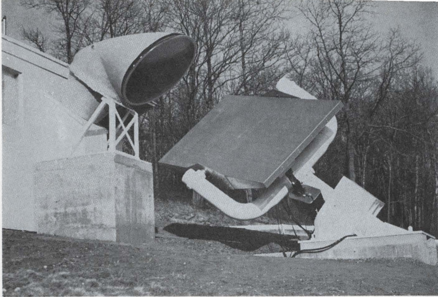
Follow the sun. The 45-square-foot mirror, right, automatically follows the sun as it moves across the sky. The other equipment, left, gathers data on how rain effects the received signals.
