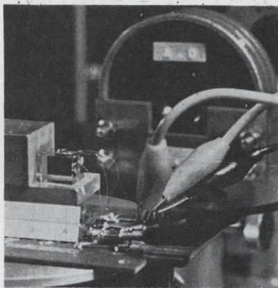
3-D. Cube of \text{TeO}_2 at center left is in optical path of laser beam coming from upper right. Acoustic transducers are attached to cube's top and side.
