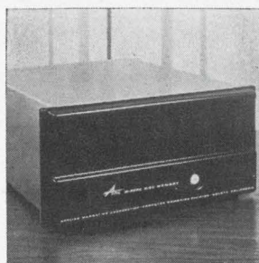
Disk memory M200C is a head-per-track type mass memory for small computers. It comes in 4 capacities ranging from 426,000 to 3,408,000 bits and average access time is 8.7 msec. Number of data tracks vary from 16 to 128 with 26,624 bits per track. Three timing racks are included, providing a bit clock, sector and origin pulse. Applied Magnetics Corp., Goleta, Calif. [388]
