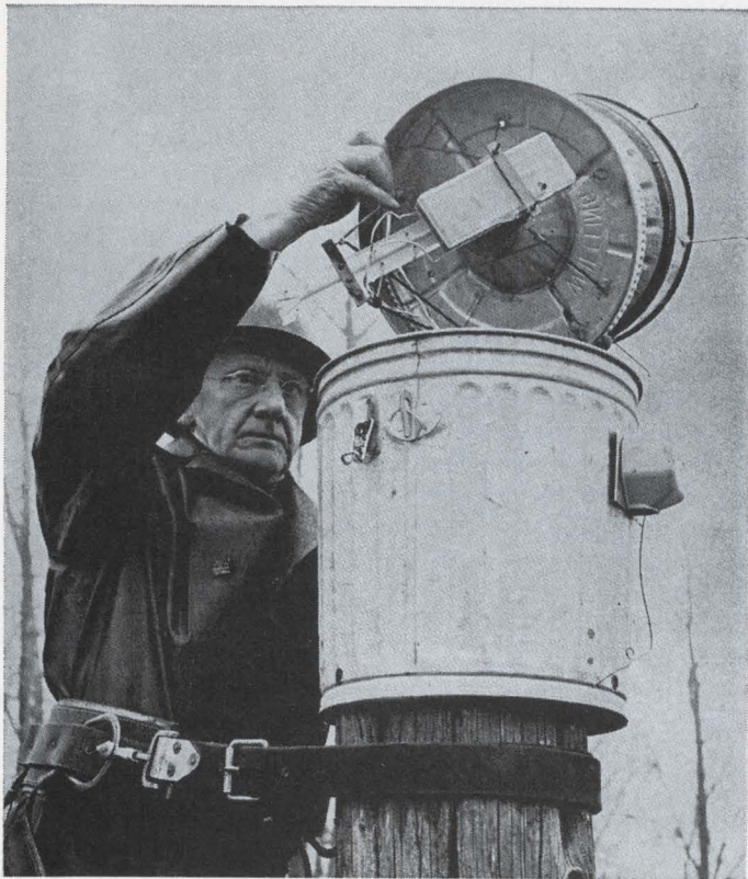
Let it rain. This modified trash can is used by Bell Labs to determine the effects of rain density on microwave transmissions. The information gathered is sent over phone lines to a computer at the labs for analysis.
