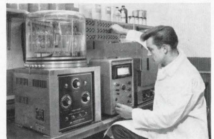
Volume and surface resistivity testing of copper-clad laminates. Exterior control unit, designed by Norplex, gives fast, reliable readout.
