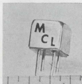
Microminiature double-balanced mixer ASK-2 covers 25 khz to 500 Mhz, occupies 0.05 cu in. Ruggedness and durability are built-in features. Internal components include precision miniature p-c boards, hot carrier diodes, and newly developed transmission line transformers. Price in quantity is under $45. Mini-Circuits Laboratory, 2913 Quentin Rd., Brooklyn, N.Y. 11229 [386]
