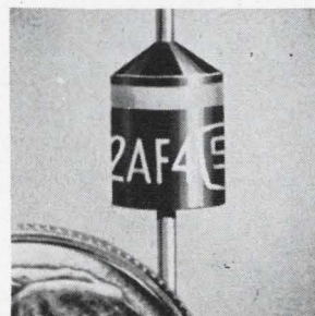
Plastic encased silicon rectifiers series 2AF have a d-c rating of 2 amps, resistive or inductive load, at 25° C and are available in 6 different piv ratings from 100 to 1,000 v d-c. Maximum rms input voltages range from 70 to 700 v d-c. All are designed to sustain peak 1 cycle surge currents of up to 60 amps. Sarkes Tarzian Inc., 415 N. College Ave., Bloomington, Ind. [442]
