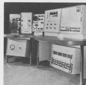
Magnetic head tester 101C is a dynamic testing unit for measuring performance of computer recording heads. It provides special circuits for simulating conditions the head undergoes when placed on a tape transport in a computer environment. Automated and manual switching is provided for studying all recording parameters. Magnetic Head Corp., Marcus Blvd., Hauppauge, N.Y. [388]
