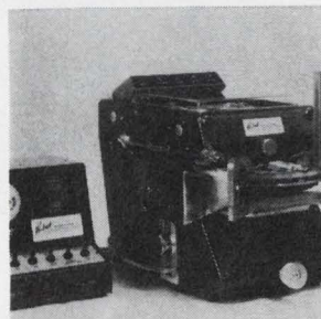
Screen printer model 1200-TT is a fully automatic machine tooled for high speed printing of conductor and resistor patterns on ceramic substrates. It screens fine lines—down to 0.003 in.—at rates up to 1,600 pieces per hour with ±0.001 in. repeatability, even on substrates with a 20% variation in thickness. Wells Electronics Inc., 1701 S. Main St., South Bend, Ind. 46623 [425]
