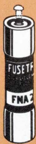
FNA FUSETRON Fuse 13/32 x 1 1/2 in. slow-blowing, Visual-Indicating, Alarm-Activating. (Also useful for protection of small motors, solenoids, transformers in machine tool industry.)
