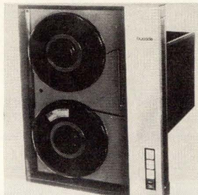
Magnetic tape system model 2045 offers industry-compatible tape recording at tape speeds to 45 in./s and packing densities to 800 b/s (non-return-to-zero, change on ones) and 1,600 b/s (phase-encoded). It features IBM tape interchangeability for either 7- or 9-track recording. Price is between $3,000 and $4,500. Bucode Inc., 175 Engineers Rd., Hauppauge, N.Y. 11787 [423]
