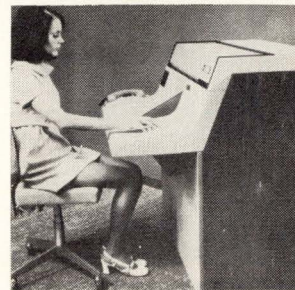
Microfilm retrieval terminal can be used in almost-real-time applications. The device incorporates a new concept in microfilm—roll microfiche—which can carry as many as 45,000 pages of computer print-out on a 100-ft. roll of 105-mm film. Prices will range from $3,750 to $7,000, depending on options. Morgan Information Systems Inc., 3197 Park Blvd., Palo Alto, Calif. [428]
