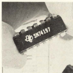
Two asynchronous TTL counters are fully programmable. The SN54/74196 decade counter and SN54/74197 binary counter are pin-for-pin replacements for the 8280/81 and 8290/91. Each counter is dc coupled, eliminating restraints normally encountered with charge-stored elements. Units count input frequencies of 0 to 50 MHz. Texas Instruments Inc., Box 5012, M/S 308, Dallas [443]
