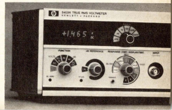
New breed. Counter (left) and rms voltmeter feature LED display and large-scale integration.
