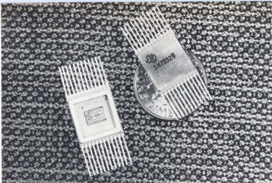
MSI TTL memory driver. from TI comes a new interface circuit for use in high-speed military memory systems.
