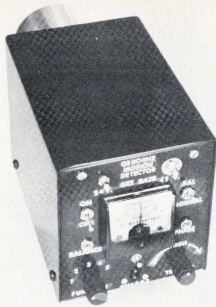
Rear view. In balance mode (switch, right), microammeter is nulled by adjusting potentiometer (above knob at left). Phase control adjusts main amplifier gain. Function knob (bottom left) is at 1 for normal operation, 2 for balancing; other positions check batteries and monitor charging. Knob, bottom right, sets triggering level of alarm.
