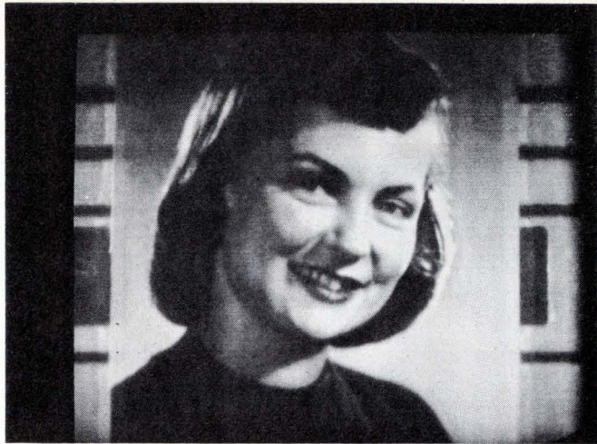
Actual scan using RL512 array. Scan rate, 2 MHz; Resolution, 6 mils; 4 bit A/D conversion provides 16 gray levels. Photo is courtesy of Recognition Equipment, Incorporated. (see Note)
