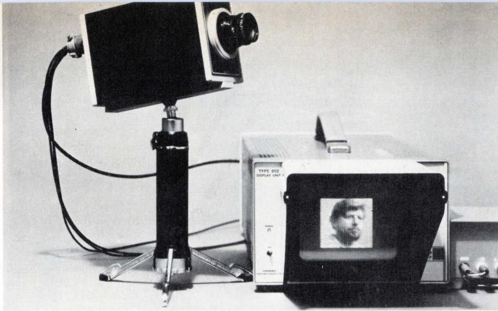
5. Image systems. Both MOS and CCD imaging arrays can be used in area imaging systems. CCD cameras potentially are capable of TV-quality resolution. MOS arrays, like this one from Reticon, are useful for lower-resolution systems.
