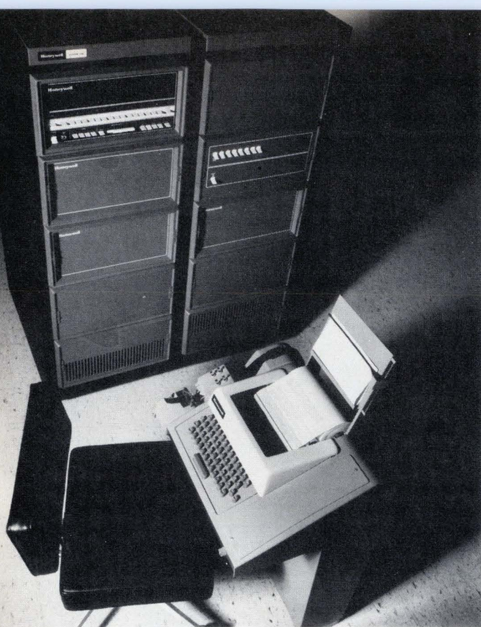
Message switch. In complex communications networks, the message switch analyzes data messages to determine their proper routing, then forwards them to other points in the network. The medium-size switch shown is based on Honeywell's H-716 minicomputer. Other panels in the rack contain line adapters, automatic calling units, and an interface to the teleprinter control unit.
