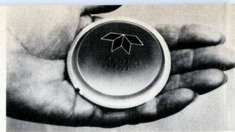
Handful. Teledyne Systems' microcomputer is 2.5 in. in diameter and sells for $1,000.
