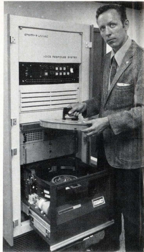
Voicebox. The heart of Univac's voice-response system is a Univac 1616 mini-computer with an audio-output section. The system is being tested by the FAA.
