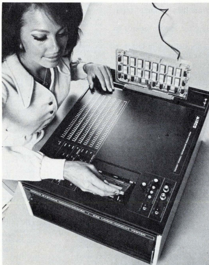
Loading test program. Magnetic-tape cassette is one of four vehicles for loading test program into logic-board tester.
