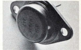
The first 3-amp positive IC regulator.
