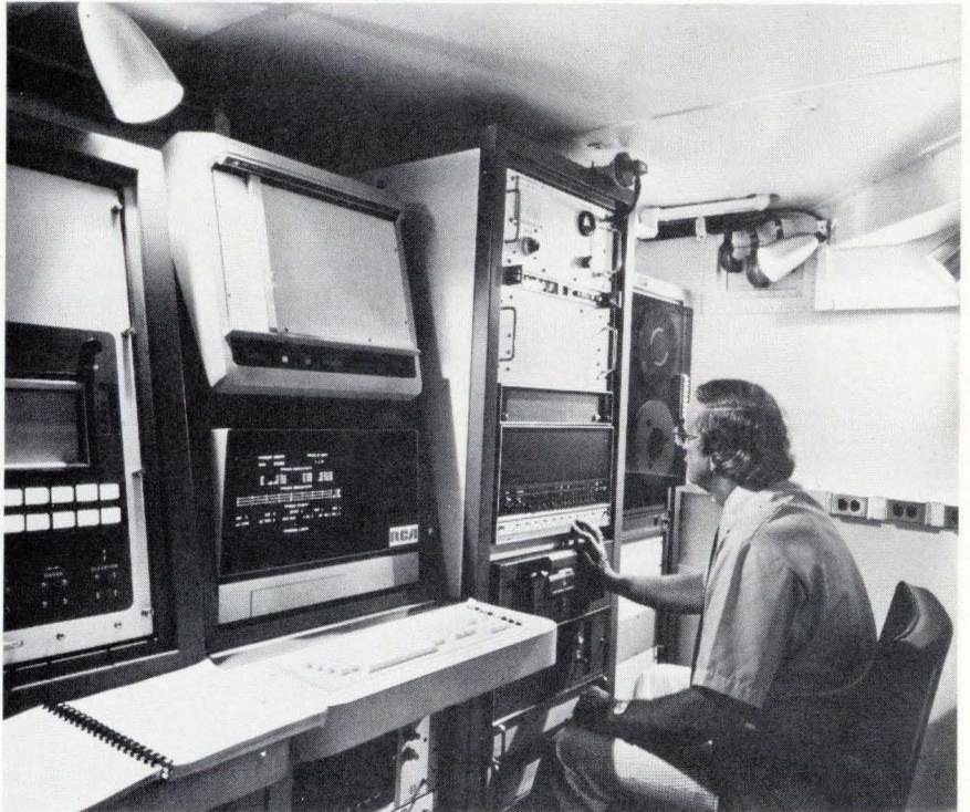
Tracker. RCA technician Charles Peterson checks out computer control of Digital Instrumentation Radar. Housed in mobile shelter, system will be used on test ranges.
