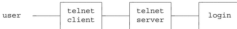
Figure 4. The tcp wrapper program has started the real telnet server and no longer participates. The user cannot notice any difference.
