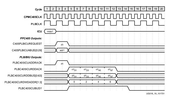
Figure 2-12: ISPLB 2:1 Core-to-PLB Line Fetch
