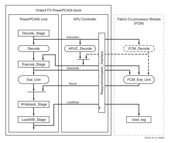
Figure 4-1: Pipeline Flow Diagram
