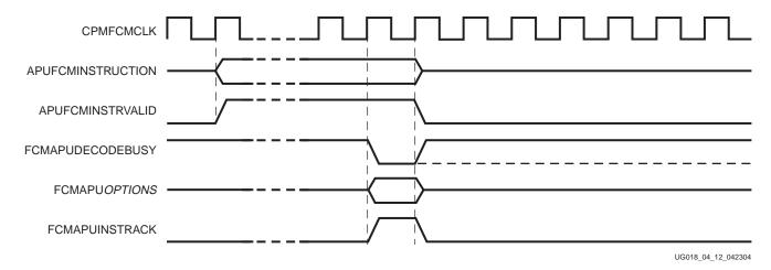
Figure 4-13: FCM Deasserting DecodeBusy
