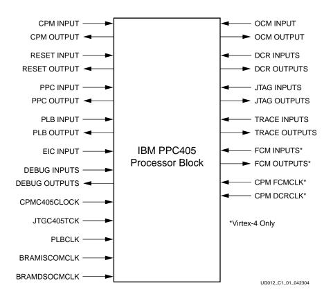
Figure C-1: PowerPC 405 Processor Block (Simplified)
