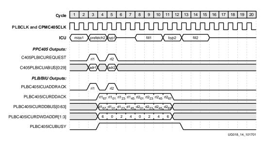
Figure 2-9: ISPLB Pipelined Cacheable Sequential Fetch (Case 2)
