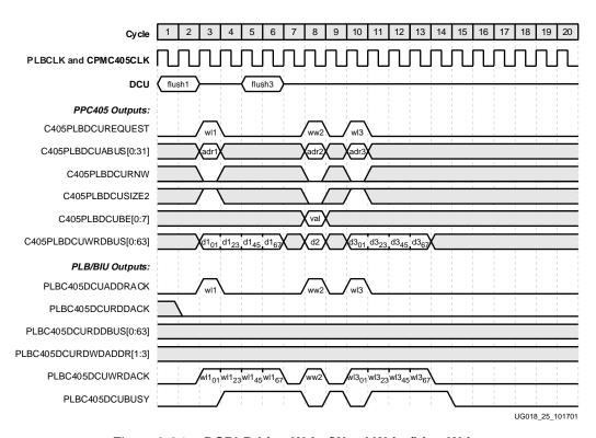
Figure 2-21: DSPLB Line Write/Word Write/Line Write
