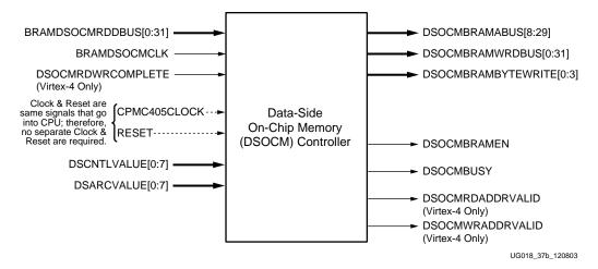
Figure 3-2: DSOCM Interface for Virtex-4
