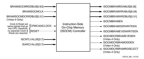
Figure 3-8: ISOCM Interface for Virtex-4
