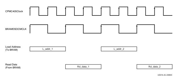
Figure 3-23: Multi Cycle Mode (2:1) Data Load Timing
