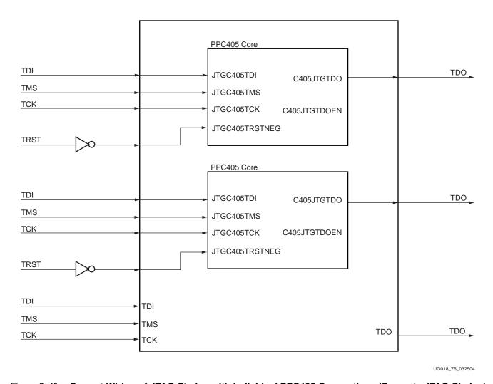
Figure 2-42: Correct Wiring of JTAG Chains with Individual PPC405 Connections (Separate JTAG Chains)
