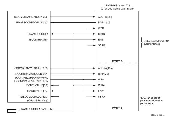
Figure 3-9: ISOCM to BRAM Interface: 8 KByte Example in Virtex-II Pro
