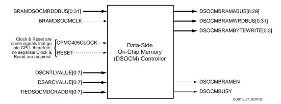
Figure 3-3: DSOCM Interface for Virtex-II Pro
