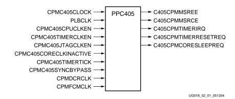
Figure 2-1: CPM Interface Block Symbol
