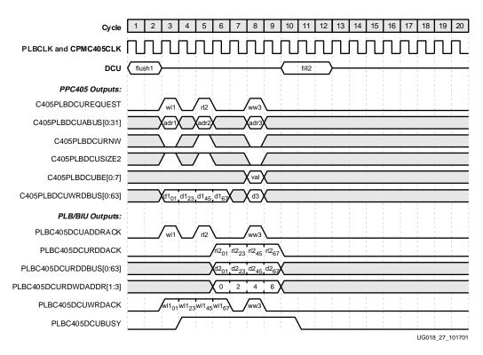
Figure 2-23: DSPLB Line Write/Line Read/Word Write
