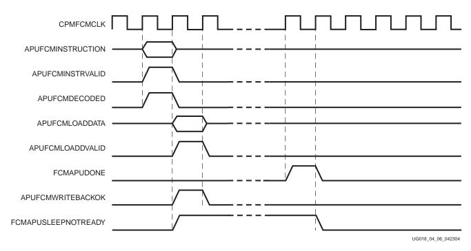
Figure 4-7: APU Controller Decoded Load Instruction Example
