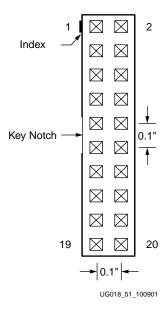
Figure A-2: Trace-Connector Physical Layout
