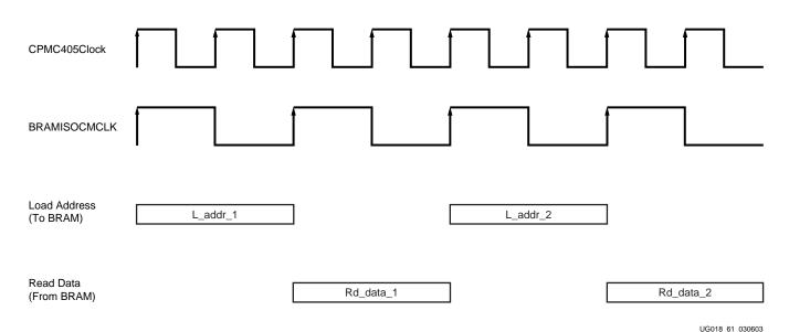
Figure 3-19: Multi-Cycle Mode (2:1) Instruction Fetch Timing
