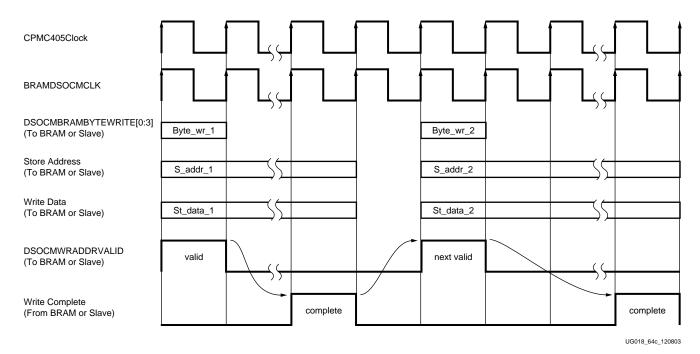
Figure 3-28: Single Cycle Mode (1:1) DSOCM Write Variable Latency Virtex-4
