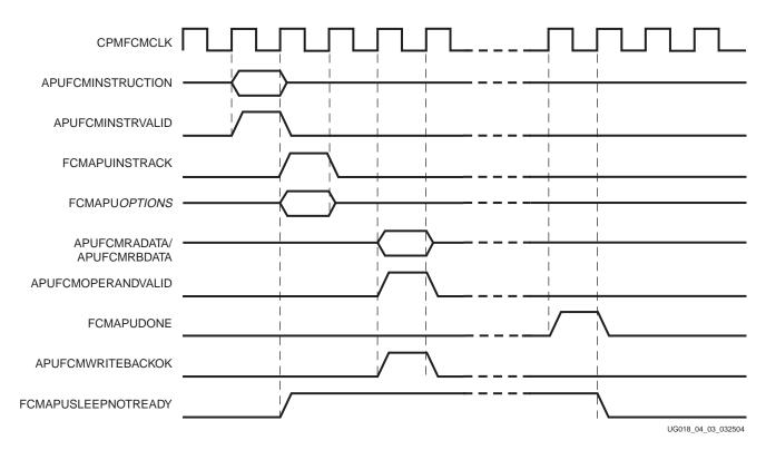
Figure 4-4: FCM Decoded Autonomous Transaction Example
