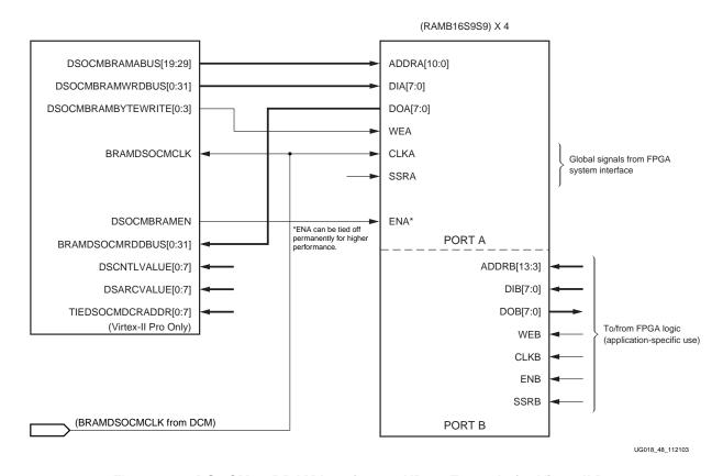
Figure 3-4: DSOCM to BRAM Interface: 8-KByte Example for Virtex-II Pro
