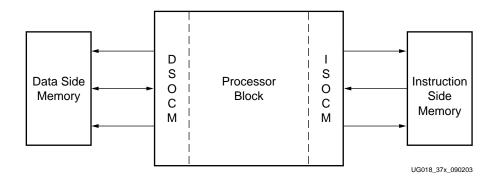
Figure 3-1: OCM Controller Interfaces
