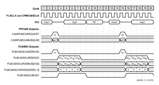
Figure 2-6: ISPLB Non-Pipelined Cacheable Sequential Fetch (Case 1)
