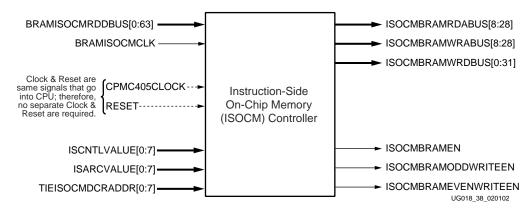
Figure 3-7: ISOCM Interface for Virtex-II Pro
