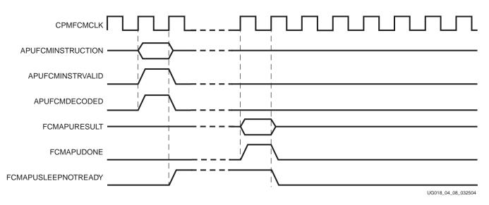
Figure 4-9: APU Controller Decoded Store Instruction
