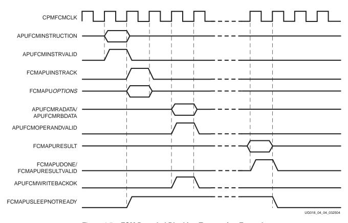
Figure 4-5: FCM Decoded Blocking Transaction Example
