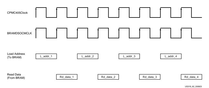
Figure 3-22: Single Cycle Mode (1:1) Data Load Timing
