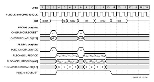
Figure 2-7: ISPLB Non-Pipelined Cacheable Sequential Fetch (Case 2)
