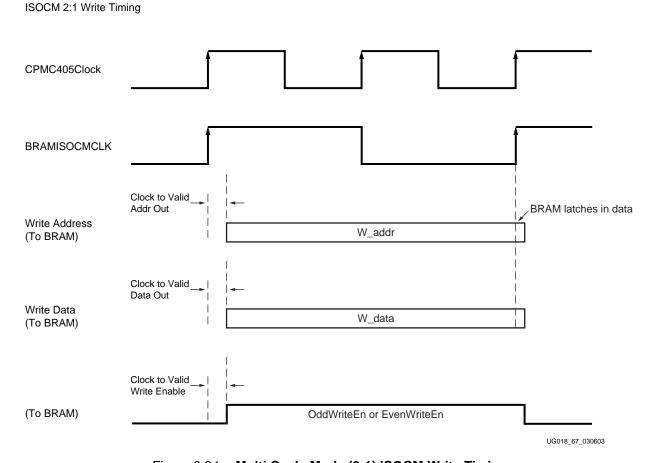
Figure 3-21: Multi Cycle Mode (2:1) ISOCM Write Timing
