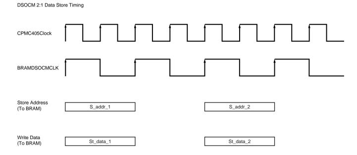
Figure 3-25: Multi Cycle Mode (2:1) Data Store Timing
