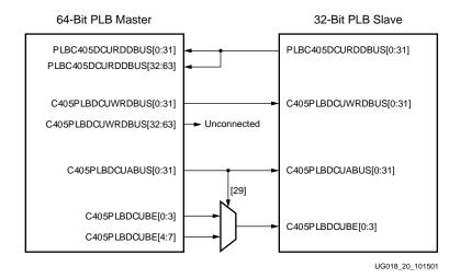
Figure 2-16: Attachment of DSPLB Between 32-Bit Slave and 64-Bit Master
