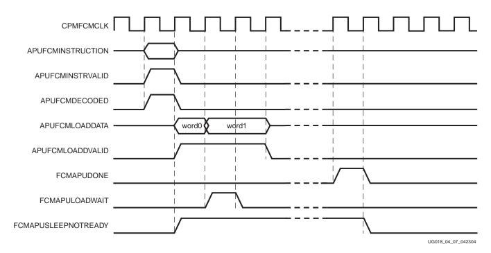
Figure 4-8: APU Controller Decoded a Double Word Load Instruction with LoadWait Example
