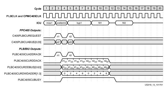
Figure 2-8: ISPLB Pipelined Cacheable Sequential Fetch (Case 1)
