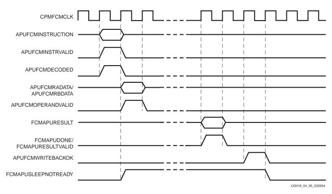
Figure 4-6: APU Controller Decoded Non-Blocking Transaction Example
