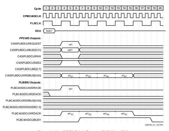
Figure 2-27: DSPLB 3:1 Core-to-PLB Line Write
