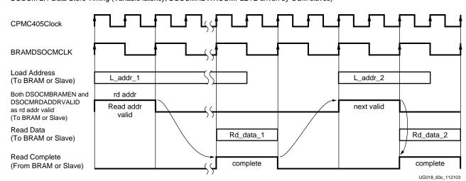
DSOCM 2:1 Data Store Timing (Variable latency, DSOCMRDWRCOMPLETE driven by OCM slaves)
