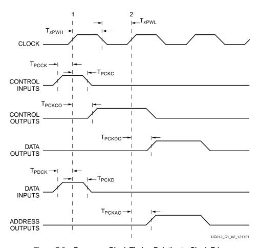
Figure C-2: Processor Block Timing Relative to Clock Edge
