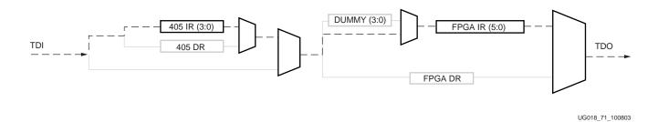
Figure 2-40: Instruction Register Data Path for Series PPC405 JTAG Connection
