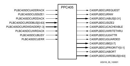
Figure 2-15: Data-Side PLB Interface Block Symbol
