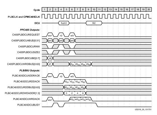
Figure 2-25: DSPLB Word Write/Line Read/Line Write
