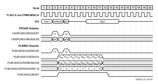
Figure 2-11: ISPLB Pipelined Non-Cacheable Sequential Fetch
