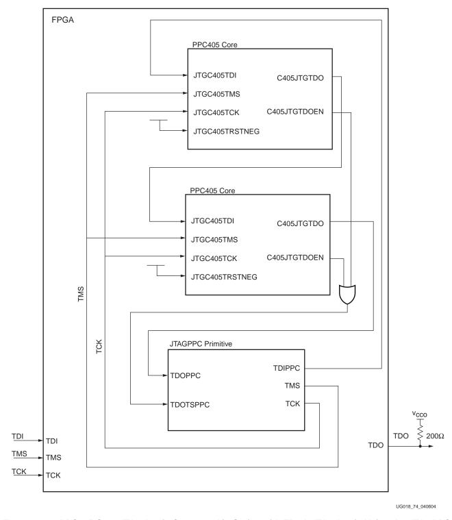
Figure 2-45: PPC405 Core JTAG Logic Connected in Series with FPGA JTAG Logic Using the JTAGPPC Primitive
