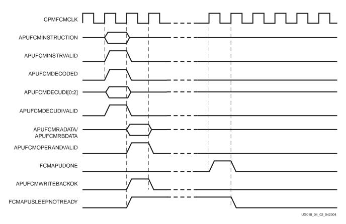
Figure 4-3: APU Controller Decoded Autonomous Transaction Example
