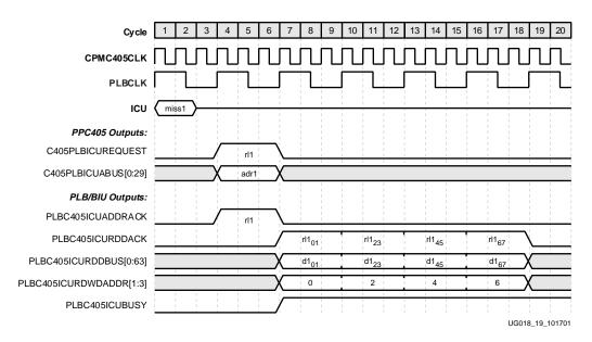
Figure 2-13: ISPLB 3:1 Core-to-PLB Line Fetch
