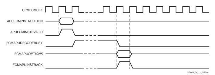
Figure 4-12: FCM Decode Asserting DecodeBusy
