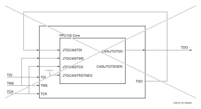
Figure 2-41: Incorrect Wiring of JTAG Chain with Individual PPC405 Connections
