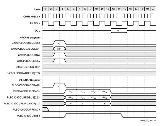
Figure 2-26: DSPLB 2:1 Core-to-PLB Line Read
