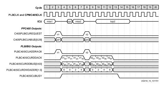
Figure 2-10: ISPLB Non-Pipelined Non-Cacheable Sequential Fetch
