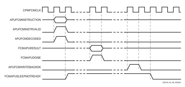
Figure 4-10: APU Controller Decoded Store Instruction with StoreWBOK=1
