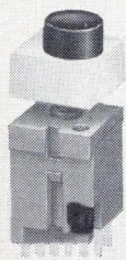
Plug-in Encoding Switches with up to eight output bits in each. Up to 256 possible code combinations may be set up within the switch using simple encoding strips. Electrical monitor and delayed strobe. Wide variety of button color combinations.
