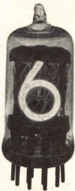
8754—Also available with right- and/or left-hand decimal points; Interchangeable with NL840/8754. Decimal-point types interchangeable with NL841, 842, 848.
