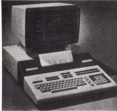
Hewlett-Packard's System 45 integrates keyboard, CPU, 64k main memory, 12" CRT, and tape input/storage media in compact computer that is based on BASIC language to provide rapid solutions for user problems
