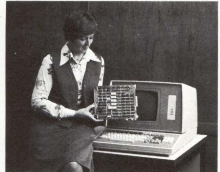
3. It has an expandable memory Display-4K RAM (4000 Characters) Program-Up to 4K PROM or 7K ROM -Up to 48K RAM
