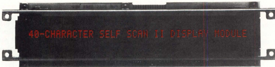
Fig 6 Plasma matrix display. Plasma display uses 5 x 7 dot matrix for alphanumerics. Similar arrangements can also be used for graphics (Photo courtesy of Burroughs Corp)
