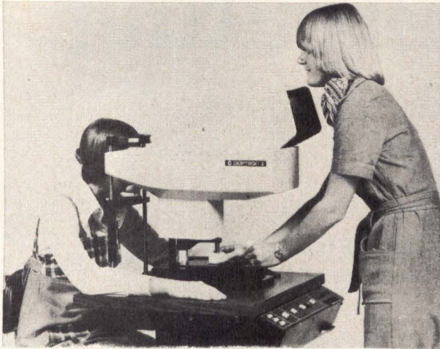
Microcomputer-controlled Diopton II in use. Only required operator adjustments are in aligning instrument to each of patient's eyes by moving joystick. Infrared imaging system, which is invisible to patient, allows operator to determine when eye is centered on target. Operator then pushes start button to initiate measuring procedure. Computer directs lenses to move in various patterns necessary to obtain at least six sequential measurements. All circuit boards and power supply are in cabinet behind switch panel
