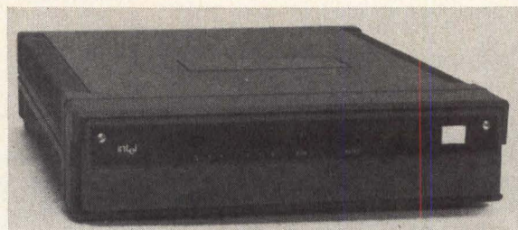
Low cost, 4-slot chassis model 210 is minimum system required for rapid development of microcomputer software. Built-in interface allows connection to user's terminal. Option permits upgrading to diskette-based system
