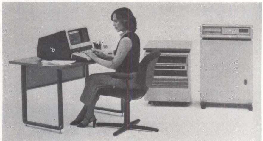
Hewlett-Packard's application of SOS technology in its 3000 family compatible series 30 reduces power and cooling requirements as well as package size
