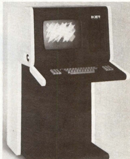
Eagle-1 graphics computer. Compact workstation can be reconfigured for different applications using standard MULTIBUS compatible peripherals.
