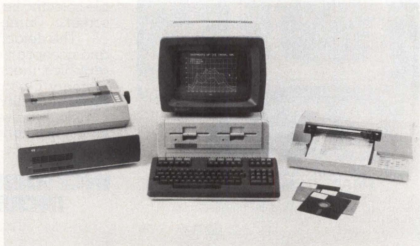
In desktop package, A600 microsystem integrates up to 3M bytes of main memory with mini-floppy and mass storage, terminal, and hardcopy output. System supports realtime networking and graphics software.
