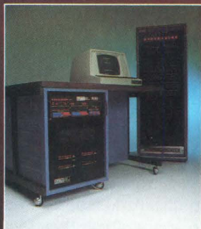
ITS (Intelligent Test System) tests up to 100 units in simultaneous operation.
