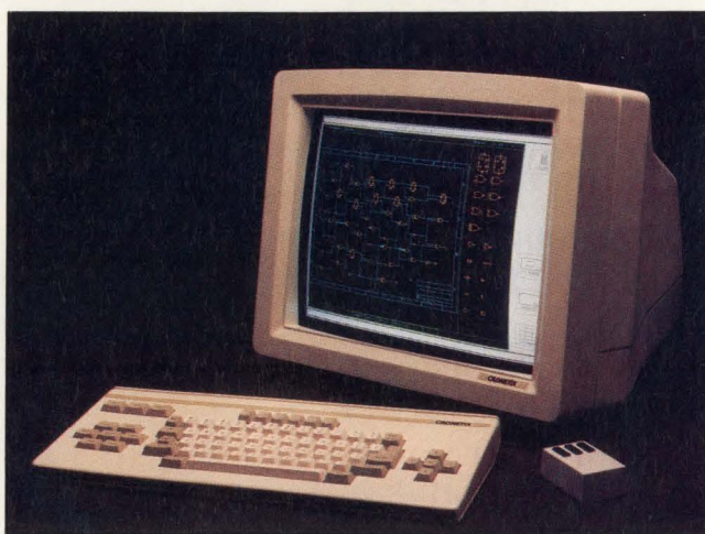
The trend toward 32-bit microprocessors to support advanced engineering workstations can be seen in machines such as the CDX500 from Cadnetix. Aimed at PC board design applications, system features include a 32-bit microcomputer, up to 3.5M bytes of main memory, and 40M bytes of Winchester disk drive memory. A 19" CRT display provides high resolution.
