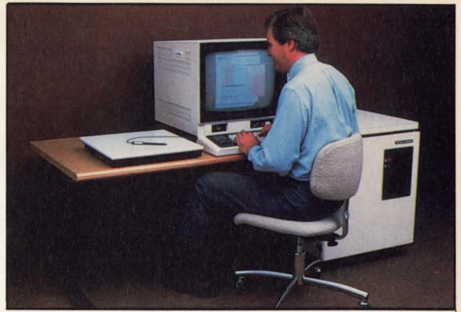
Apollo Computer's DN600 Domain workstation fits into a LAN of dedicated 32-bit computational nodes connected by coax cable. Each workstation contains VLSI CPU, memory, 19" color graphics monitor, separate keyboard, and graphics processor; optional peripherals are also available.
