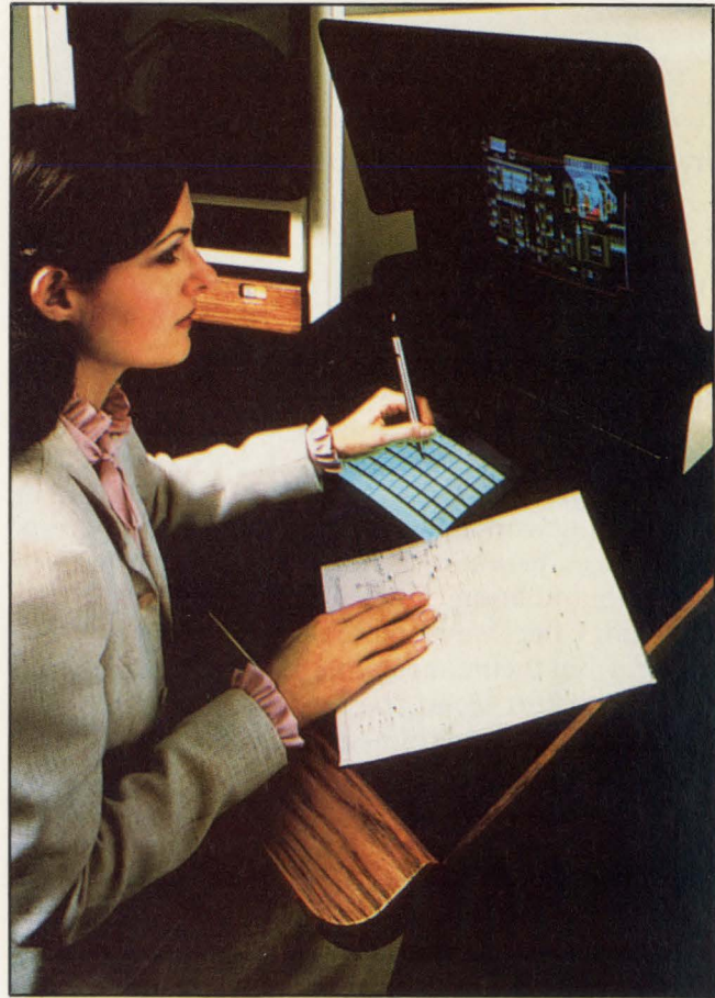
User interface with the Telesis Systems' workstation is simplified by a lightpen interactive CRT display. Called the “function screen,” this display emulates functions that might require five separate functions on other workstations.
