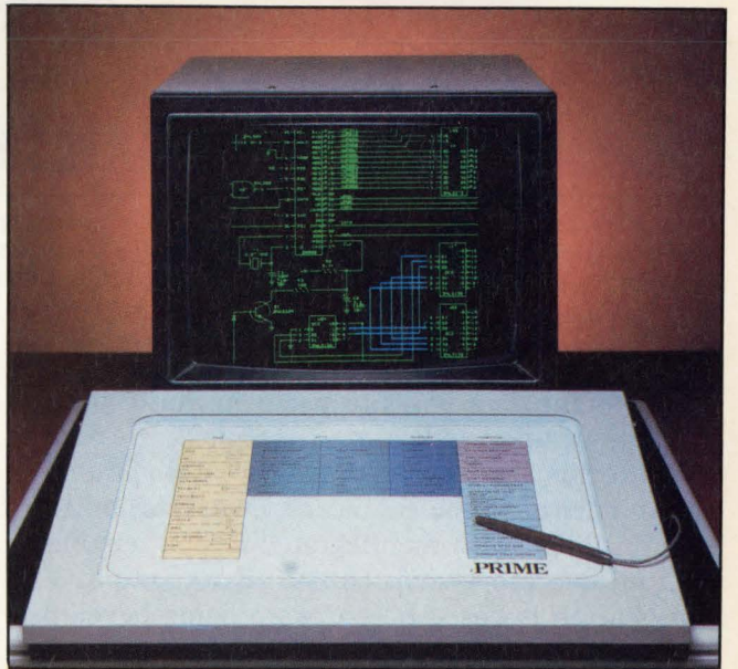
Powerful CAD/CAM systems, such as Prime Computer's Electronic Design Management System (EDMS) depend on equally powerful computers like that company's 32-bit 50 series. The menu-driven, multi-user engineering workstation can handle all aspects of interactive digital logic design and drafting.
