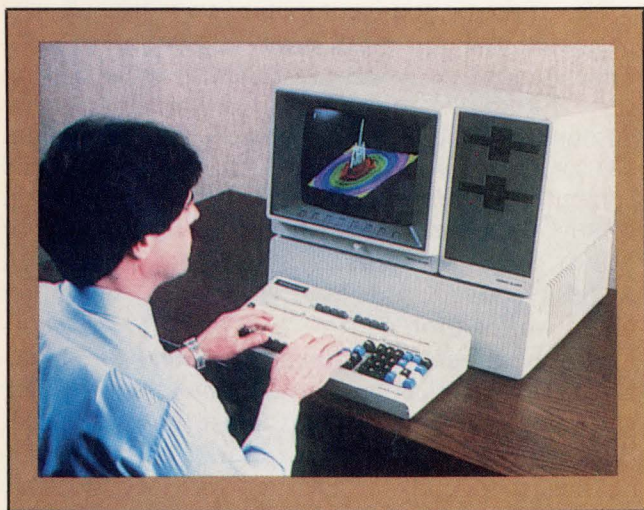
The model 7500 scientific computer, based on the Motorola MC68000 microprocessor, is available in both color and monochrome versions. Each Perkin-Elmer workstation includes two 5¼" floppy disk drives, the Unix-like IDRIS operating system, two RS-232 ports, ASCII keyboard, full-feature BASIC interpreter, and keyboard overlay.
