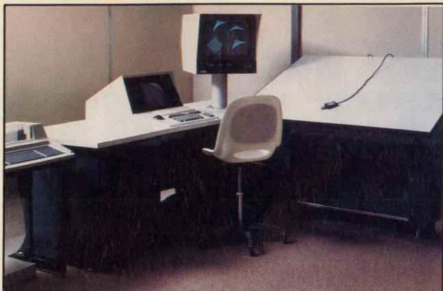
Advanced engineering workstations such as the AYCAD from Aydin can just about do it all. This turnkey system runs on the CP/M operating system and includes many features. Separate microprocessors run the system's digitizer tablet and graphics vector generator.
