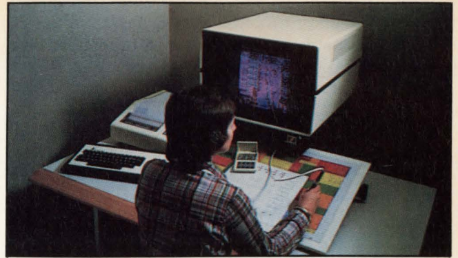
Computervision's Instaview interactive design workstation can be used for a variety of CAD/CAM applications. A wide range of specialized software capabilities plus PCB and integrated circuit design significantly increase the designer's productivity.
