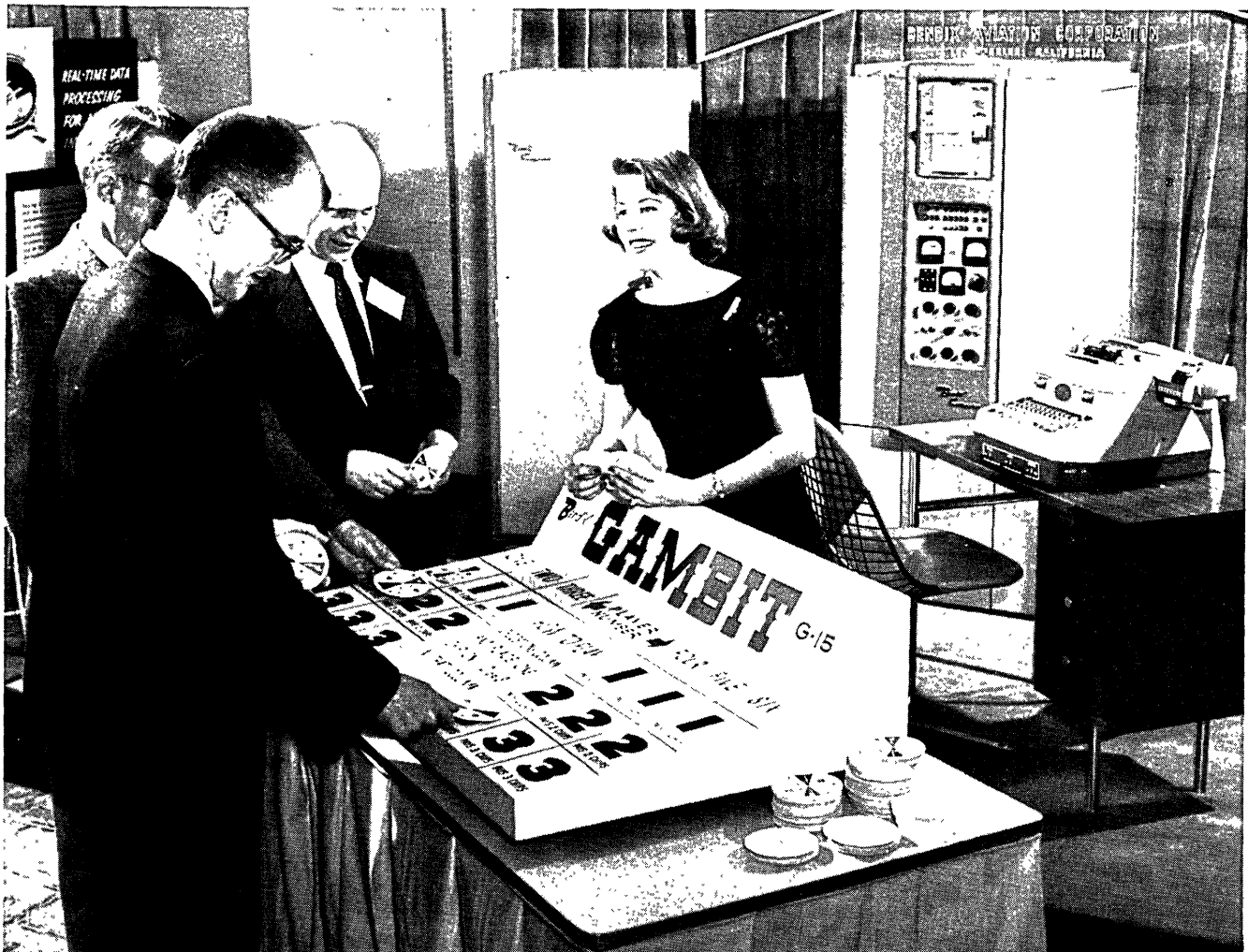
ELECTRONIC ROULETTE, "GAMBIT", a game devised by engineers of the Bendix Aviation Corporation's Computer Division to illustrate the company's newest general purpose computer. When all of the jumbo "chips" are down, the attendant flicks a switch, the computer calculates the odds and automatically types out the winning number.
