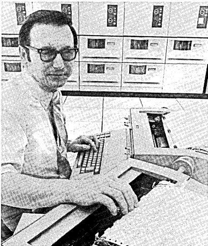
— Dr. Walter Jacobs, a blind colleague at the laboratory, examines the Braille output from an experimental embossing terminal
