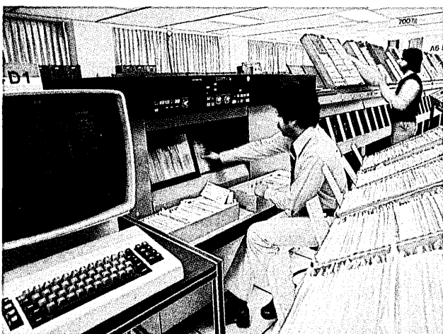
At Wells Fargo Bank, operators work with one of eight IBM 3890 Document Processors. Each machine can read and sort over 2,000 MICR encoded documents a minute.
