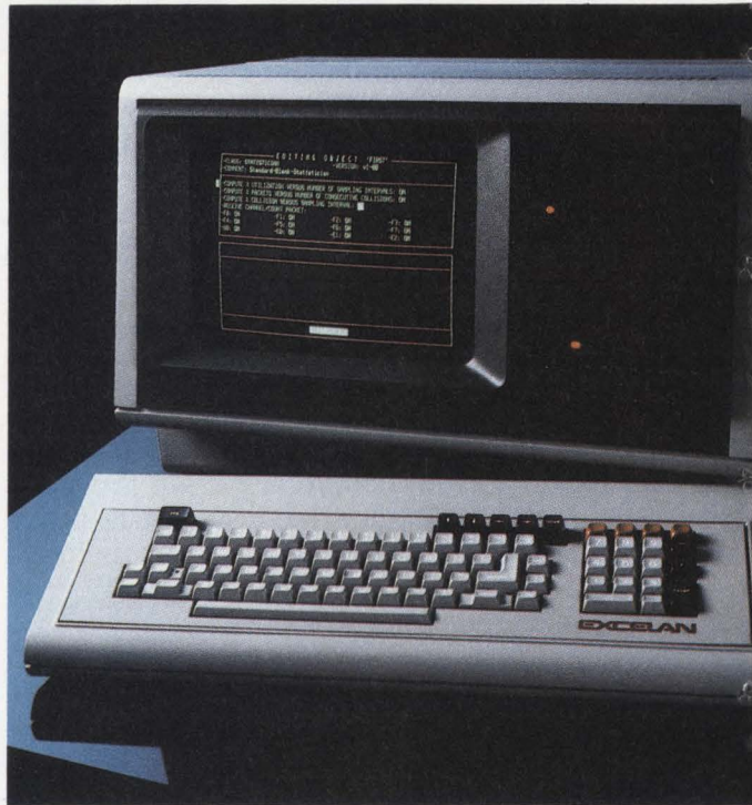
Figure 8: The Excelan Nutcracker provides extensive monitoring and control functions by simulating actual network usage.
